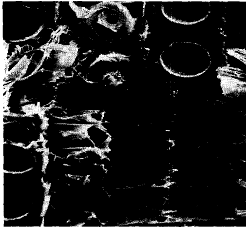
FIG. 2. Scanning electron micrograph of a radial surface of Douglas-fir, showing ray cells between two layers of vertical tracheids.
