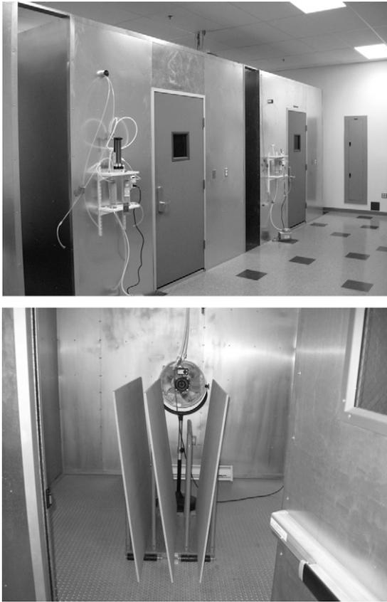
Figure 1. Typical large-chamber testing facility at a California Air Resources Board-approved third-party certifier (top photo: exterior of large chambers with air sampling apparatus shown at the Composite Panel Association testing facility in Leesburg, VA; bottom photo: interior of large chamber with samples loaded for testing).
