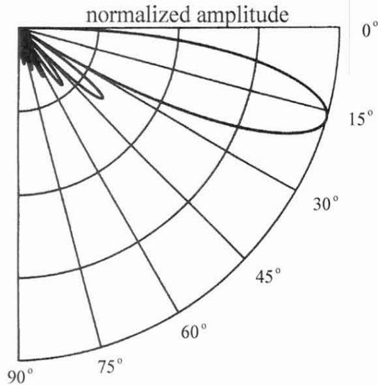
FIG. 6. Profile of a critically refracted longitudinal wave in an isotropic medium. Adapted from Langenberg et al. (1990). Used with permission.
