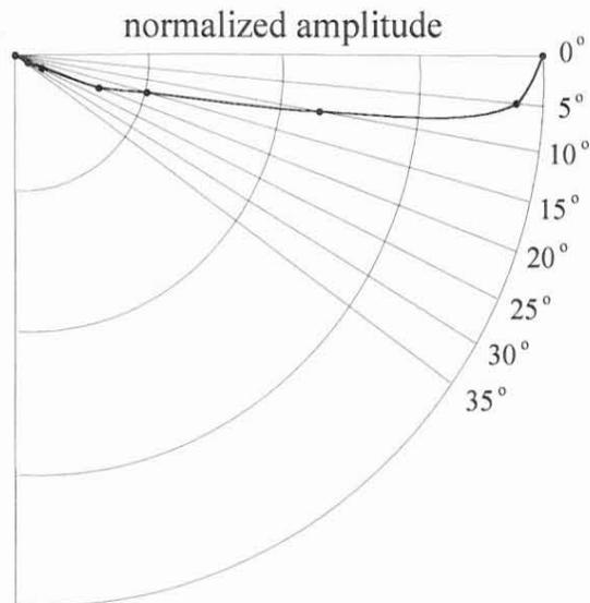
FIG. 4. Profile of critically-refracted longitudinal wave in Block A (GRA =  $90^\circ$ ). Wood is flatsawn with respect to the wide face.
