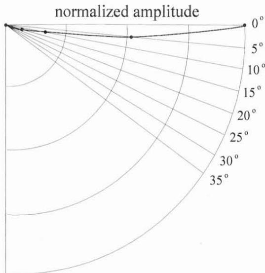
FIG. 5. Profile of critically refracted longitudinal wave in Block B (GRA =  $0^\circ$ ). Wood is quartersawn with respect to the wide face.
