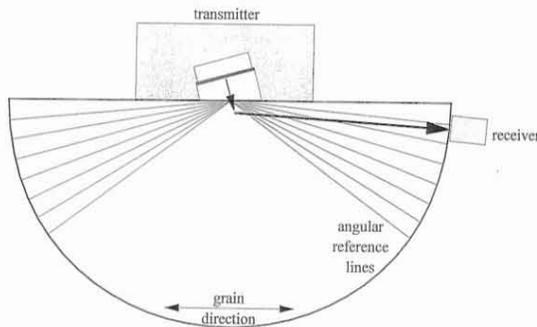
FIG. 2. Beam profile setup.
