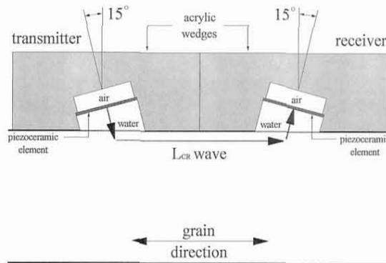
FIG. 1. Pitch-catch transducer arrangement for ultrasonic inspection of pine using  $L_{CR}$  waves.
