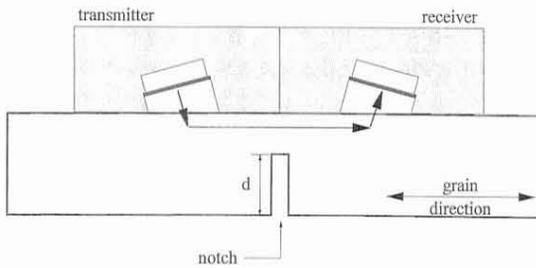
FIG. 3. Beam depth-of-penetration setup.
