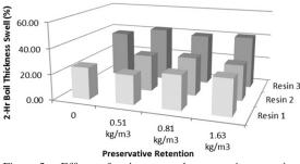
Figure 2. Effects of resin type and preservative retention on 2-h boil thickness swell of aspen flakeboard.
