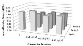
Figure 1. Effects of resin type and preservative retention on internal bonding strength (IB) of aspen flakeboard. (resin 1 =phenol-formaldehyde resin [PF]; resin 2 = PF [85]/ soy hydrolysate [15] blend resin; resin 3 = PF-crosslinked soy resin).
