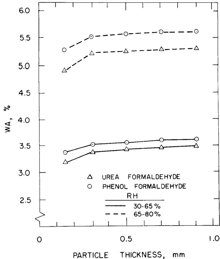
FIG. 3. Predicted effect of particle thickness and changes in relative humidity (RH) on the water adsorption (WA) of particleboard with a specific gravity of 0.70.
