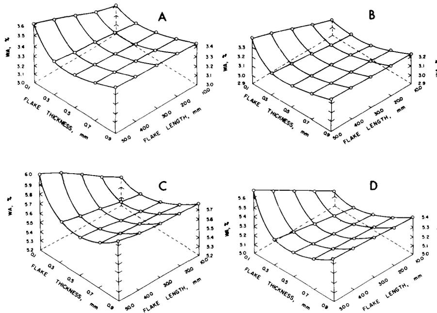
FIG. 1. Predicted effect of flake length and thickness on the water adsorption (WA) of flakeboard (specific gravity = 0.70) when relative humidity changes (A) from 30–65% in a PF-bonded board, (B) from 30–65% in a UF-bonded board, (C) from 65–80% in a PF-bonded board, and (D) from 65–80% in a UF-bonded board.
