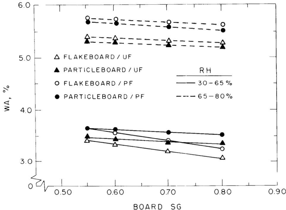
FIG. 2. Predicted effect of board specific gravity (SG) and changes in relative humidity (RH) on the water adsorption (WA) of flakeboard made with 0.30- × 50-mm flakes and particleboard made with particles 0.40 mm thick.
