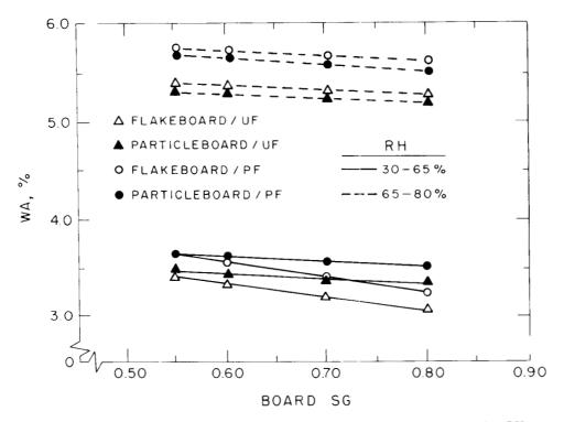
FIG. 2. Predicted effect of board specific gravity (SG) and changes in relative humidity (RH) on the water adsorption (WA) of flakeboard made with 0.30-  $\times$  50-mm flakes and particleboard made with particles 0.40 mm thick.
