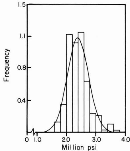
FIG. 2. Two-hundred 30-inch segment MOE values measured from 50 boards were used to form the histogram. A normal distribution fit is superimposed over the histogram.
