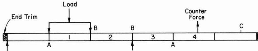
FIG. 1. Location of the four 30-inch segments for flatwise MOE measurements and loading configuration for segment 1 are shown. For segment 2, supports are at points A, load at points B, and counter force at point C. To test segments 3 and 4, the specimen was turned end for end in the equipment. Load was applied perpendicular to the wide face of the specimen.
