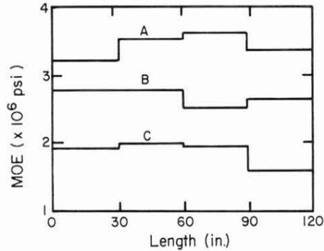
FIG. 3. The lengthwise variability in MOE as measured on a 30-inch span is shown for three specimens of the 2 x 4 MSR lumber.
