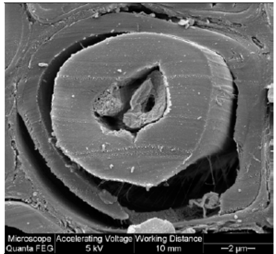
Figure 3. High resolution environmental scanning electron microscopy image of a G-layer in the fiber lumen of Kwila wood (taken by environmental scanning electron microscopy in Canada).
