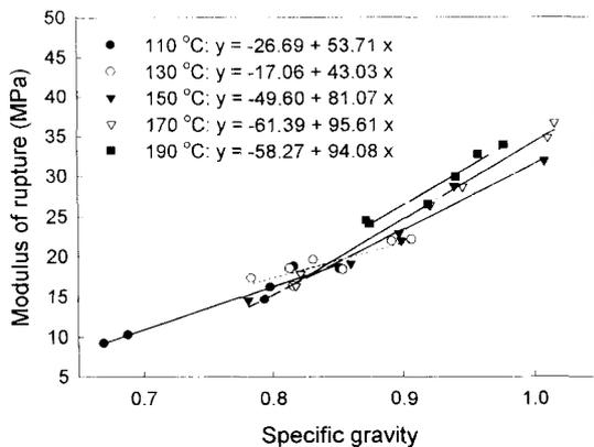
FIG. 3. MOR vs. SG for wood fiber/polymer fluff composites processed at different press temperatures.
