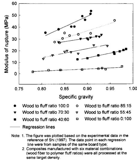
FIG. 1. MOR vs. SG for wood fiber/polymer fluff composites manufactured with different material combinations.
