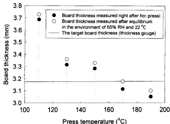
FIG. 2. Thickness springback of the wood fiber/polymer fluff composites processed at different press temperatures.
