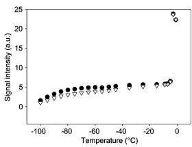
Figure 12. Bulk magnetic resonance signal intensity vs temperature as the black spruce sapwood sample froze: original data (•) and corrected for temperature ( $\bigtriangledown$ ) as defined by Curie's Law. Carr Purcell Meiboom Gill measurement was undertaken. An abrupt phase change of free water occurred at  $-3^{\circ}$ C. A second phase change (bound water) was observed below  $-60^{\circ}$ C.
