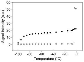
Figure 13. Bulk signal intensity of bound ( $\bullet$ ) and free (o) water vs temperature from the corrected data of Fig 12 as the black spruce sapwood sample froze. Carr Purcell Meiboom Gill measurement was undertaken. The ratio of signal from free and bound water was approximately 3:1.
