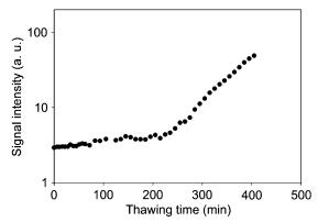
Figure 8. Semilog plot of the signal intensity of the long lifetime components (free water) of Fig 7 as a function of thawing time of black spruce sapwood. The ring boundary of thawing emerges in the sensitive volume commencing at 200 min.
