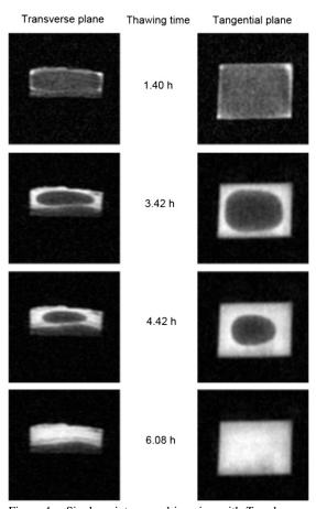
Figure 4. Single-point ramped imaging with  $T_1$  enhancement (*SPRITE*) magnetic resonance imaging of a black spruce sapwood sample in the transverse (left) and tangential (right) planes as a function of thawing time at ambient temperature. A moving ring boundary of thawing front was observed.
