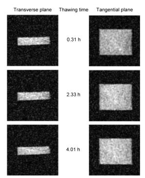
Figure 10. Single-point ramped imaging with  $T_1$  enhancement (*SPRITE*) magnetic resonance imaging of a black spruce heartwood sample in the transverse (left) and tangential (right) planes as a function of thawing time. No changes occurred even after 4.6 h of warming. The heartwood sample was at the FSP. Therefore, most of the water was in the cell walls. Bound water was not frozen at measurement conditions.
