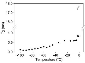
Figure 14. Bulk  $T_2$  of bound (•) and free (o) water vs temperature from the corrected data of Fig 12 as the black spruce sapwood sample froze. Carr Purcell Meiboom Gill measurement was undertaken. The  $T_2$  of bound water was much shorter than the  $T_2$  of free water.
