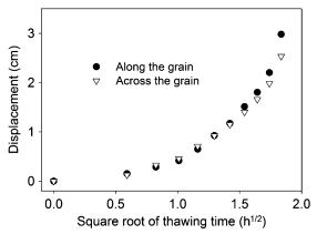
Figure 5. Displacement of the ring boundary of the thawing front both along and across the grain directions from Fig 4 as a function of the square root of thawing time. Displacement increased nonlinearly as the black spruce sapwood sample thawed. The thawing front progression was nearly identical both along and across the grain.
