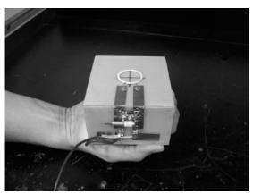
Figure 1. The unilateral magnet device used in this study. The white circle on the face of the magnet array is the radiofrequency probe. The sensor is connected to the *Bruker Minispec* console, and the radiofrequency probe is placed adjacent to the wood sample for moisture content measurements.
