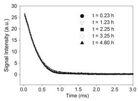
Figure 9. Time-domain bulk free induction decay (FID) signal as the black spruce heartwood sample thawed from 0.23 to 4.60 h using the Nalorac 2.4-Tesla horizontal bore superconducting magnet. The  $T_2^*$  signal lifetime was constant at 400 µs. No water phase transition was observed.
