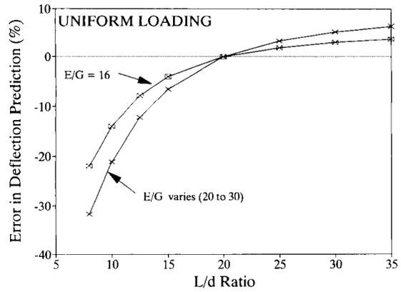
FIG. 6. Error in predicted deflections for glulam beam with uniform loading.
