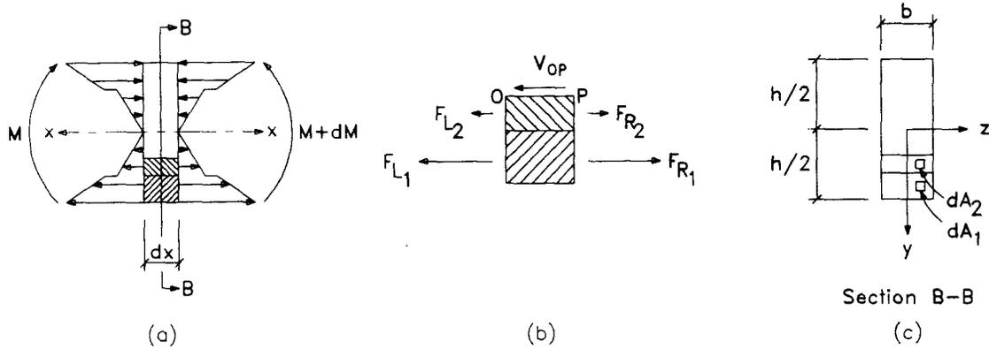
FIG. 2. Stresses, forces and moments on the composite cross section.
