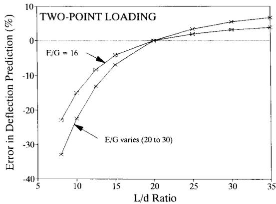
FIG. 5. Error in predicted deflections for glulam beam with two-point loading.
