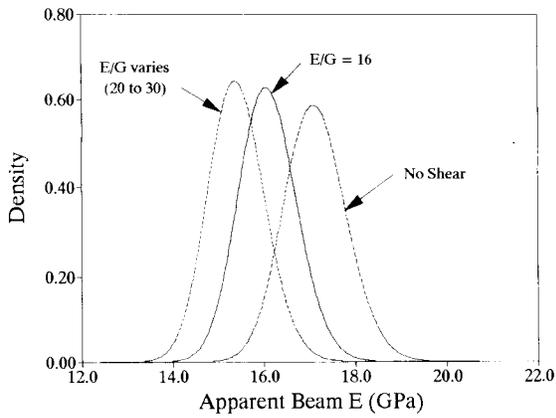
FIG. 4. Predicted probability density functions of apparent beam E for three E/G assumptions.
