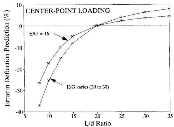
FIG. 7. Error in predicted deflections for glulam beam with center-point loading.
