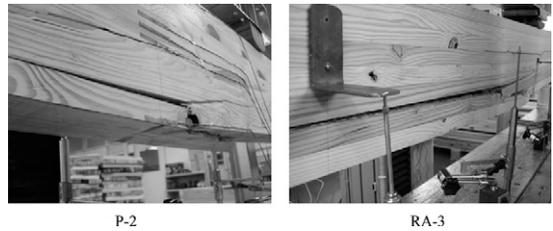
Figure 4. Failure of glue line for rejected specimens.
