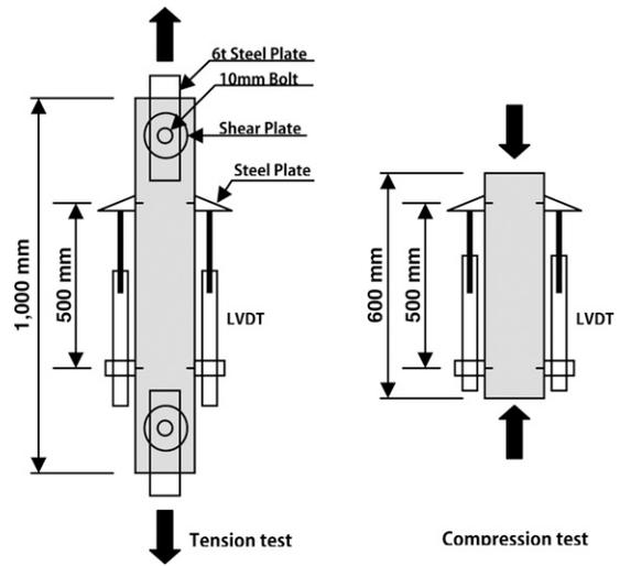
Figure 2. Configuration for tension and compression tests of actual size laminates.
