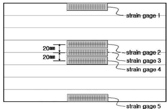
Figure 1. The location of strain gauges.
