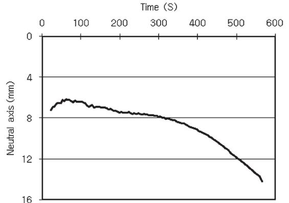
Figure 3. Neutral axis shift by time (LR-2).
