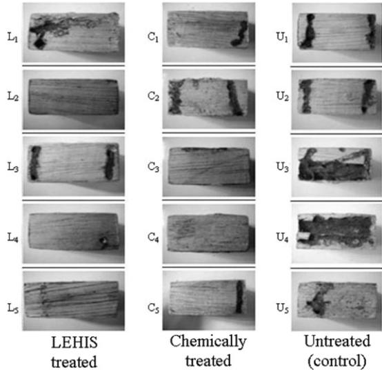
Figure 4. Actual decimations from termites on wood samples. Left column is low-energy hydrogen ion shower-treated, middle column is chemically (pyrethroid toxin) treated, and right column is untreated (control).
