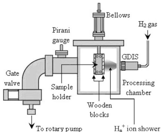
Figure 2. Schematic diagram of the overall facility.
