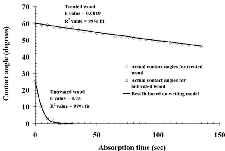
Figure 8. Numerical constructs of  $d\theta/dt = -k\theta$  (wetting model) fitted against empirical data. The time rate equation of the wetting model is made to fit actual contact angle data of treated and untreated wood samples. Low-energy hydrogen ion shower-treated sample shows lower  $k$  value compared with control. Lower  $k$  values denote longer moisture absorption time.
