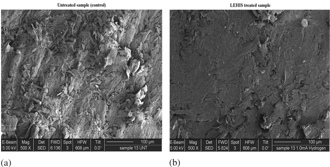
Figure 6. Typical scanning electron micrographs (5 kV, 500 $\times$  magnification) of the (a) untreated and (b) low-energy hydrogen ion shower (LEHIS)-treated samples. LEHIS irradiation caused the pores and voids on the surfaces to close.
