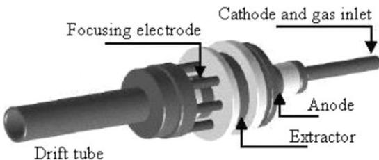
Figure 1. 3-D illustration of gas discharge ion source (GDIS).
