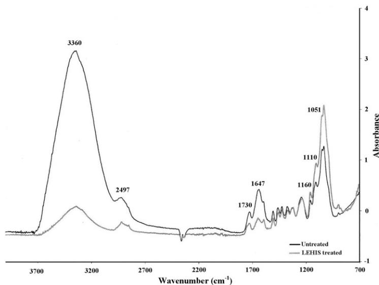
Figure 7. Fourier transform spectra of both control and treated specimens. Treated specimen shows weakening of the polar groups, thus exhibiting enhanced hydrophobic property.
