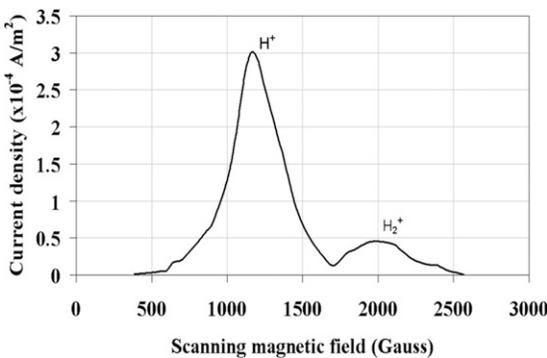
Figure 5. Typical mass spectrum of low-energy hydrogen ion shower. The ion shower consists of  $\text{H}^+$  and  $\text{H}_2^+$  ions.
