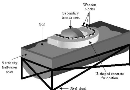
Figure 3. 3-D illustration of the subterranean termite nest.
