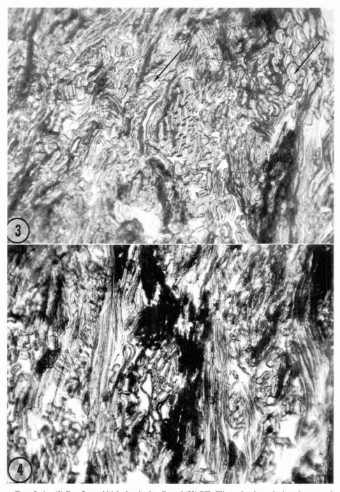
FIGS. 3, 4. (3) Dry-formed high-density hardboard (2% PF). Fibers closely packed; resin unevenly distributed; fiber lumina free of resin (arrows).  $\times 200$ . (4) Dry-formed medium-density hardboard (6% PF). Fibers less densely packed; resin densely aggregated.  $\times 200$ .
