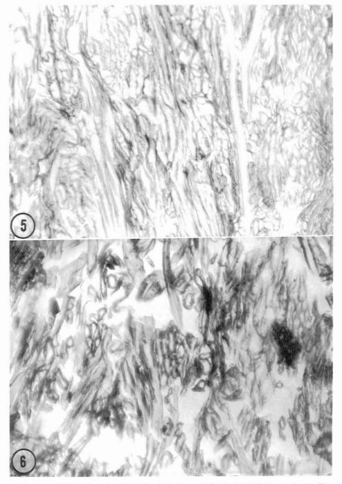
FIGS. 5, 6. (5) Wet-formed medium-density hardboard (4% PF with 0.6% Rhodamine B). Fibers closely packed; resin evenly distributed.  $\times 150$ . (6) Dry-formed medium-density hardboard (6% PF with 0.6% Rhodamine B). Fibers loosely packed; resin shows localized accumulations.  $\times 150$ .
