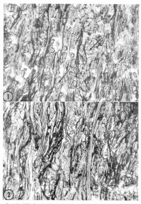
FIGS. 1, 2. (1) Wet-formed medium-density hardboard (2% PF). Fiber lumina free of resin (arrows); resin evenly distributed.  $\times 200$ . (2) Wet-formed medium-density hardboard (4% PF). Resin deposition more intense because of higher resin concentration in the board.  $\times 200$ .
