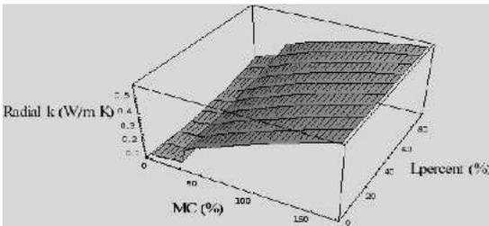
FIG. 10. Radial thermal conductivity values predicted for Scots pine for latewood percentage from 5% to 99% and MC from 0% to maximum 178%.
