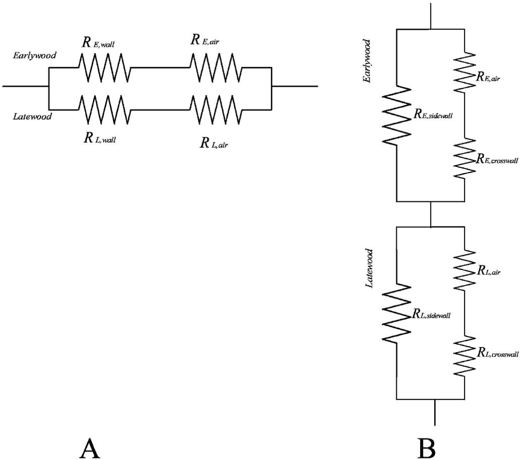
FIG. 5. Thermal resistance model for softwood species. A-tangential direction, B-radial direction.
