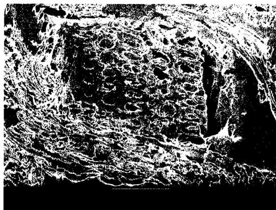
FIG. 2. Scanning electron micrograph of a block composed of composite Material A showing the intimate association between the wood and plastic, but also illustrating the presence of voids between these materials.
