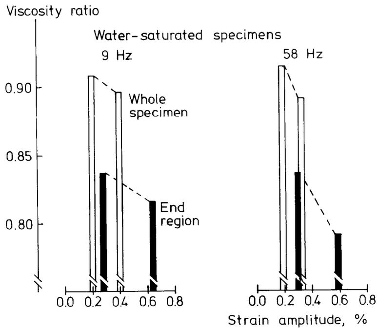
FIG. 9. Viscosity ratios of whole specimen and of the end region at different strain amplitudes. Compression conditions according to Fig. 8. The dotted lines connect specimens from the same block.
