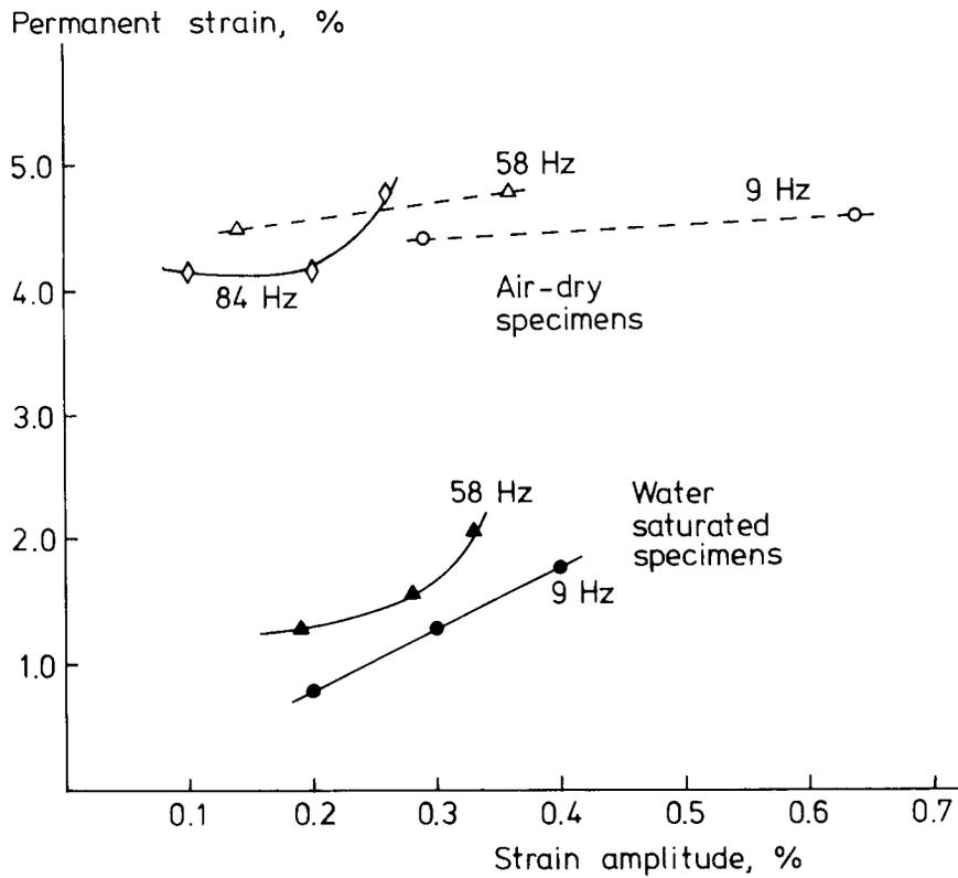
FIG. 8. Permanent strain after a compression straining of 6.5% parallel to the grain versus strain amplitude. Time of relaxation: 5 min.
