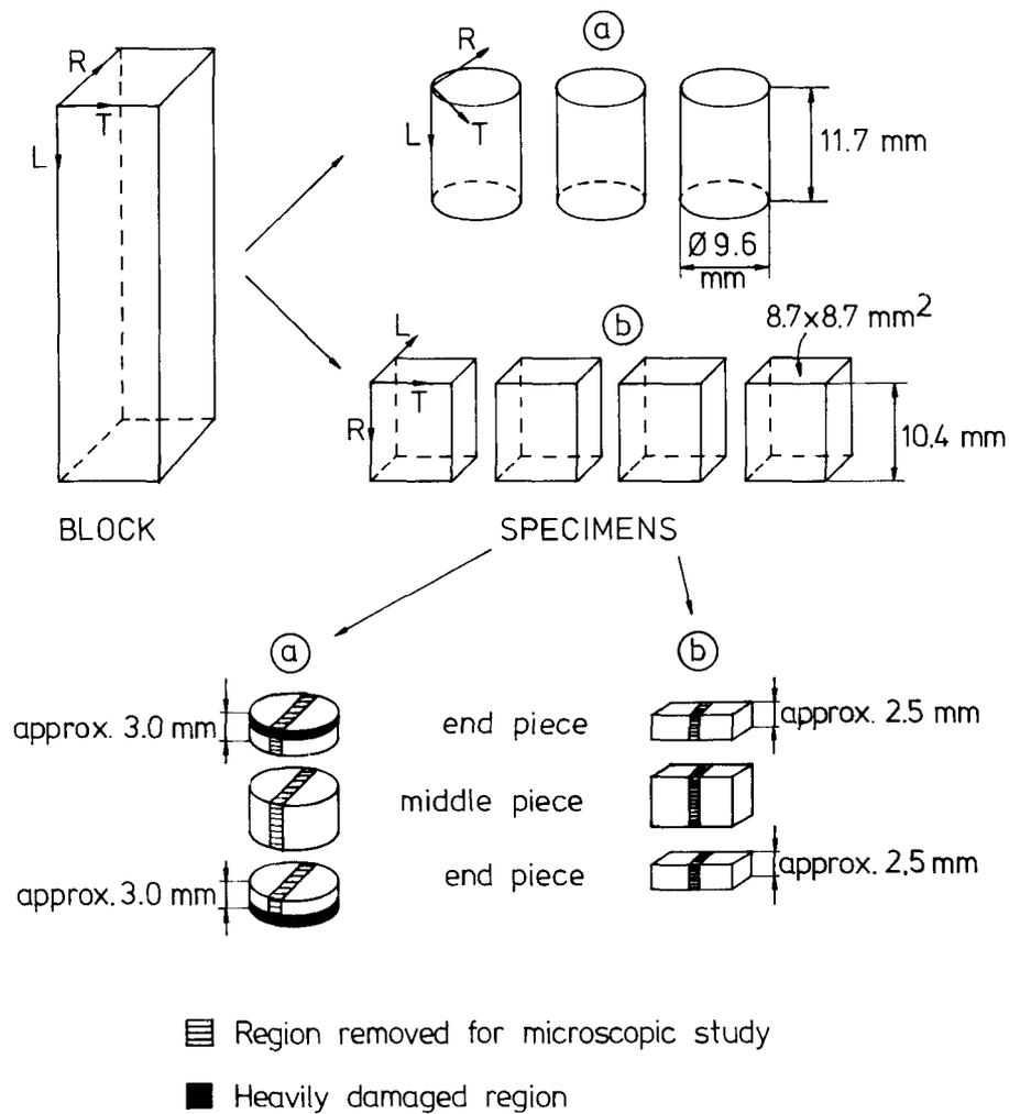
FIG. 1. Preparation and subdivision into pieces of specimens used in compression parallel to the grain (a) and perpendicular to the grain (b).
