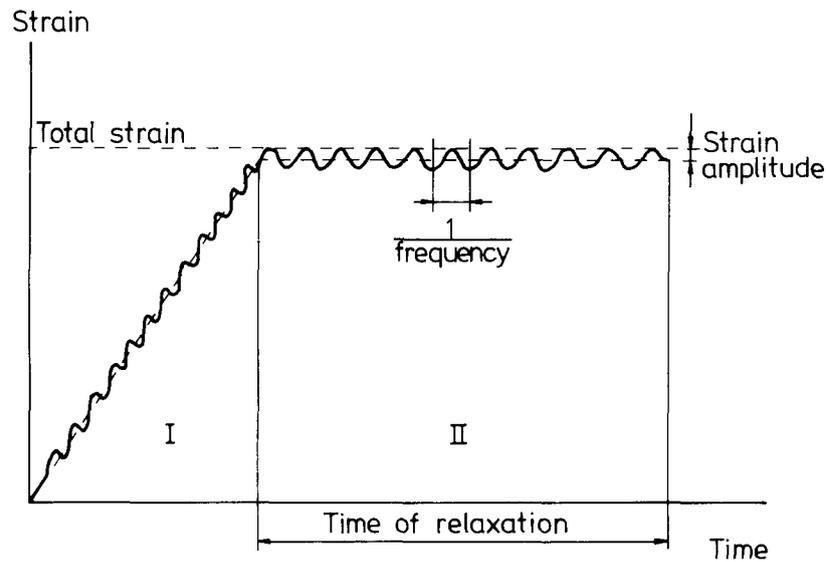
FIG. 2. Compression with superimposed small sinusoidal oscillations. I. Compression period. II. Relaxation period.
