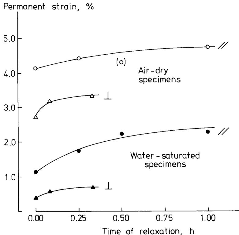
FIG. 10. Permanent strain after a compression straining of 6.5% versus time of relaxation. Strain amplitude: 0.25%. Frequency: 58 Hz. Symbols according to Fig. 6.
