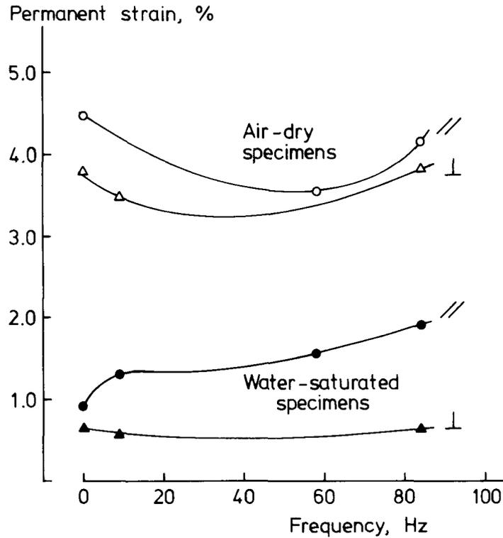
FIG. 6. Permanent strain after a compression straining of 6.5% versus frequency. Strain amplitude: 0.25%. Time of relaxation: 5 min.
