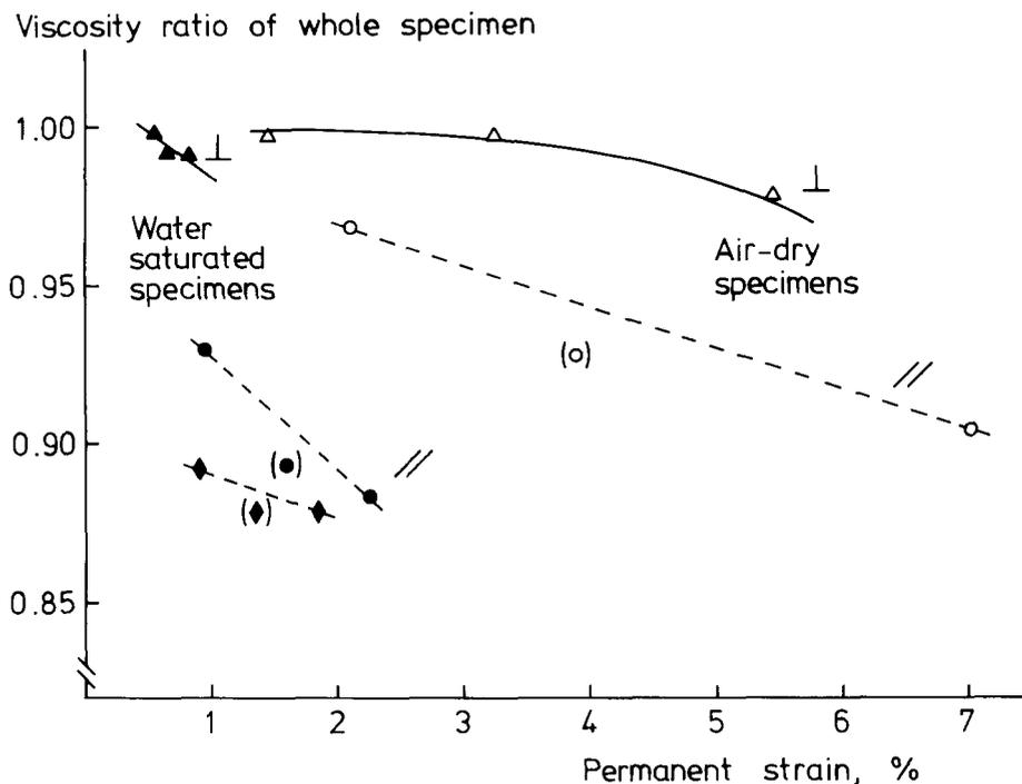
FIG. 5. Viscosity ratio of whole specimen versus permanent strain. Compression conditions according to Fig. 3.
