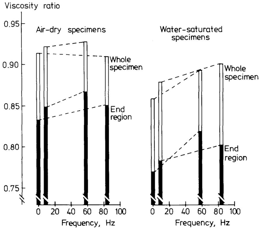
FIG. 7. Viscosity ratio of whole specimen and of the end region at different frequencies. Compression conditions according to Fig. 6. The dotted lines connect specimens from the same block.
