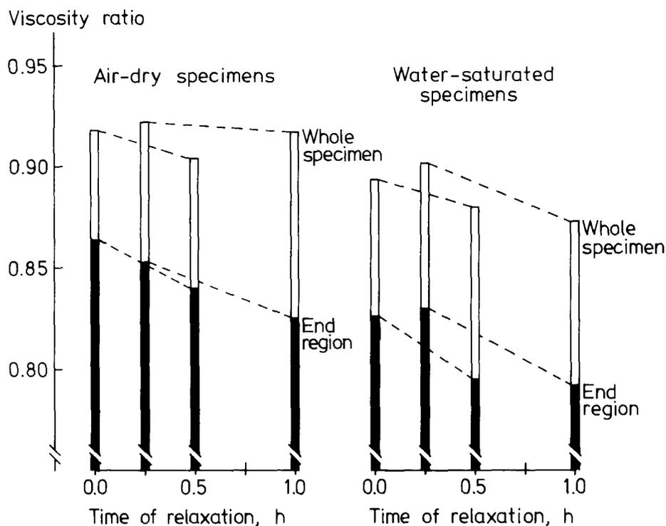
FIG. 11. Viscosity ratio of whole specimen and of the end region at different times of relaxation. Compression conditions according to Fig. 10. The dotted lines connect specimens from the same block.
