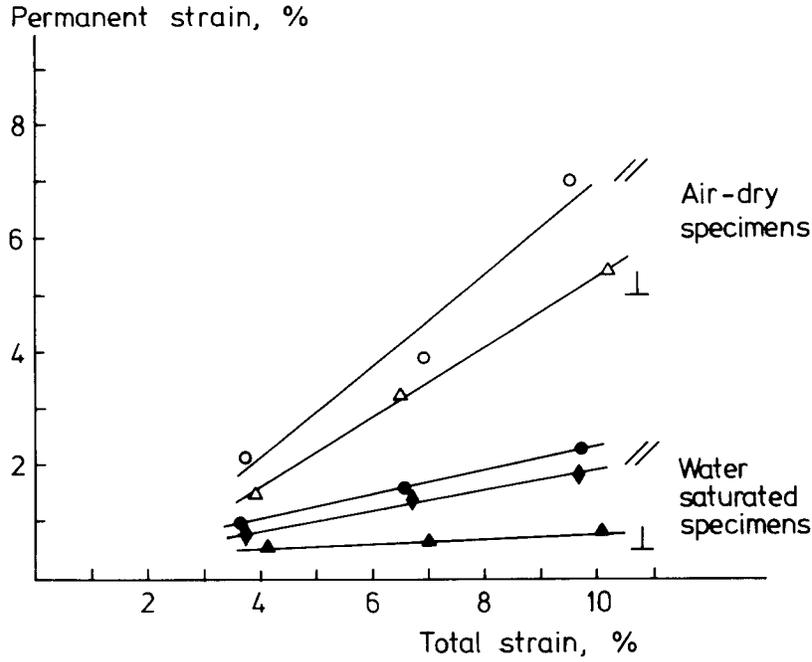
FIG. 3. Permanent strain versus total compression strain. Strain amplitude: 0.27%. Time of relaxation: 5 min.
