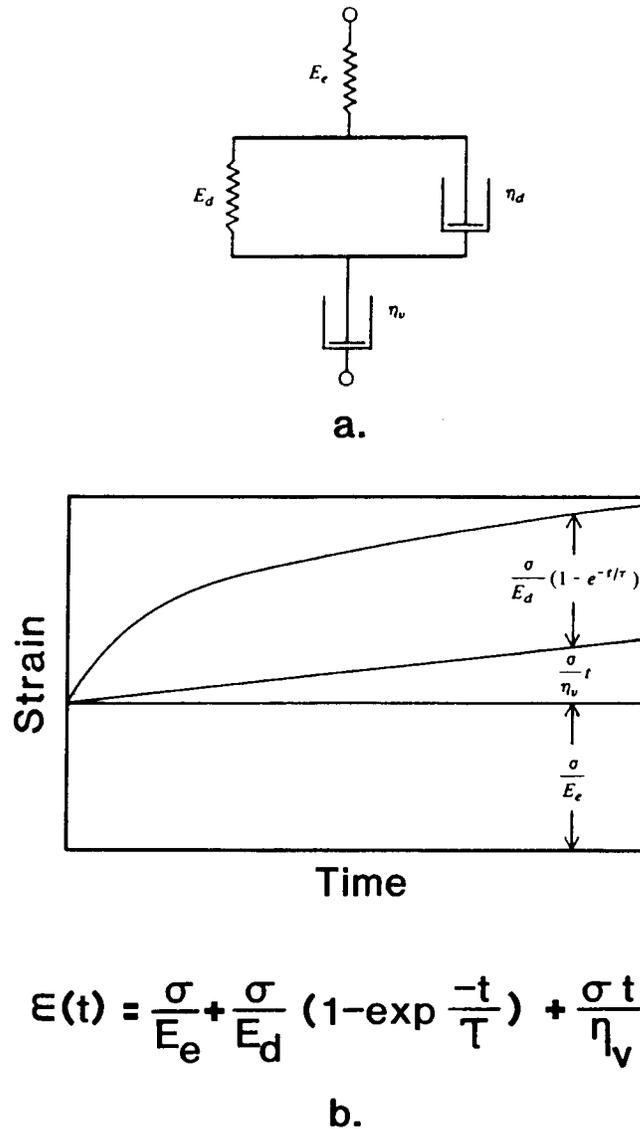
FIG. 1. (a) Four-element Burger model for creep of linear viscoelastic materials. (b) Flexural creep strain versus time as per the Burger model.
