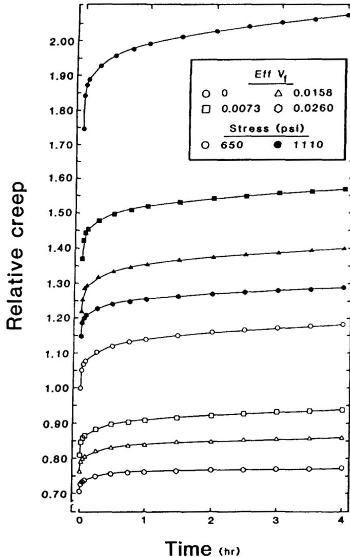
FIG. 2. Influence of effective reinforcement volume fraction ( $\text{Eff } V_f$ ) and stress level on the relative creep of glass fiber reinforced hardboard with time.
