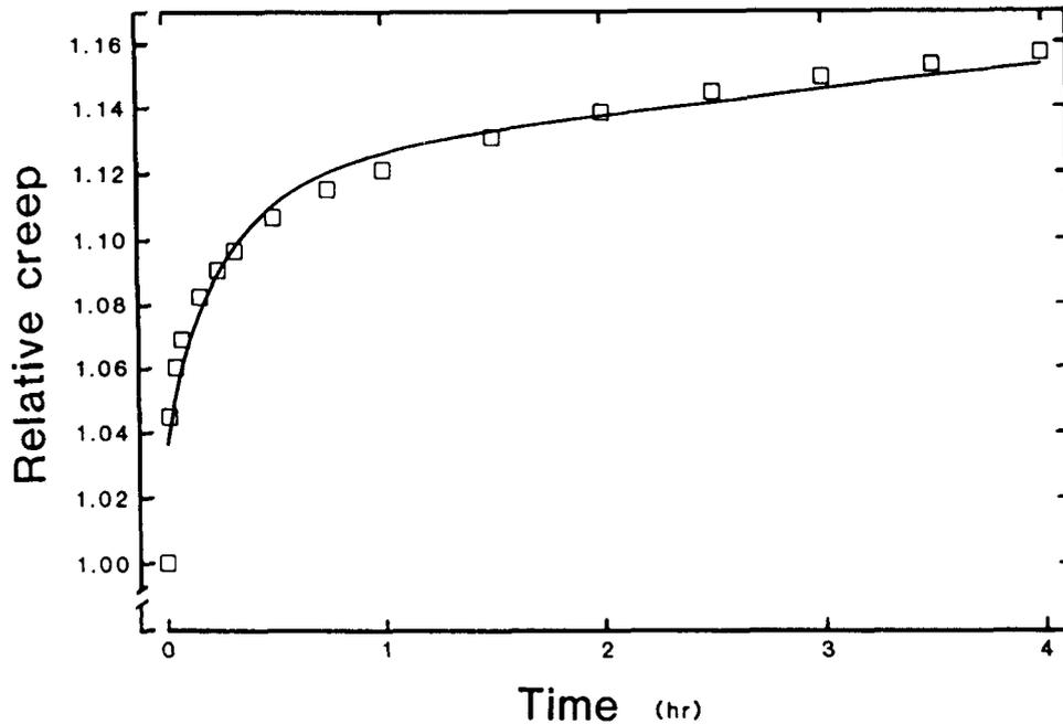
FIG. 4. Relative observed ( $\square$ ) and predicted (—) creep deflection of glass fiber reinforced hardboard at an effective reinforcement volume fraction of 0.0073 under a stress of 650 psi.
