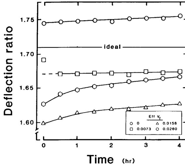
FIG. 3. Influence of effective reinforcement volume fraction ( $\text{Eff } V_f$ ) on the creep deflection ratio of glass fiber reinforced hardboard with time. The deflection ratio is equal to the observed deflection under a stress of 1,110 psi divided by the deflection observed under a stress of 650 psi. A deflection ratio of  $1,110/650 = 1.71$  represents ideal linear viscoelastic behavior.
