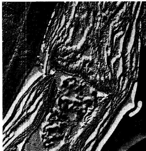
FIG. 6. Exploded cell walls of ray parenchyma in ammoniated compression wood. Transverse section. 4820 $\times$
