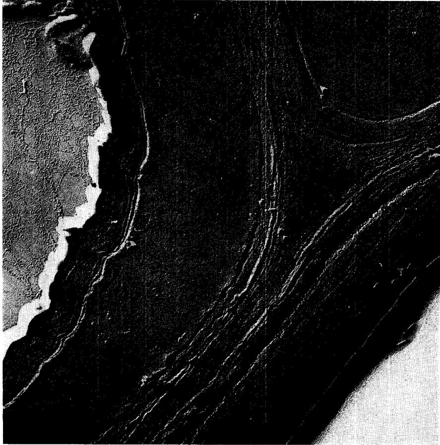
FIG. 3. Transverse section of ammoniated earlywood. Note crimpings in S3 layer. 10750 $\times$
