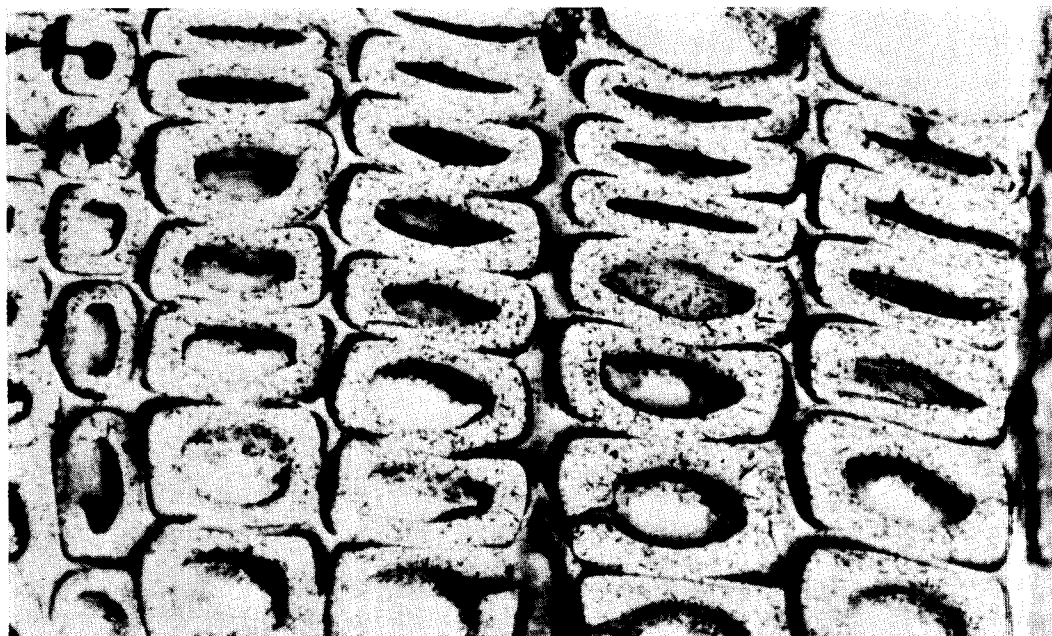
FIG. 1. Bright field autoradiograph of uncoated spruce exposed to tritiated water vapor. The middle lamella regions contain less tritium than the cell walls. 600 \times .
