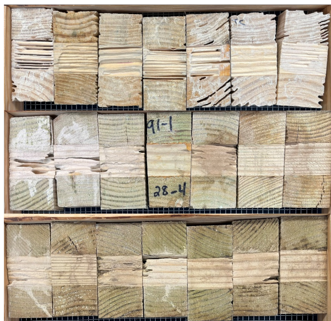
Figure 6. Cross-laminated timber 3-ply: (a) untreated, (b) MCA-treated, and (c) CA-C-treated samples following exposure to Reticulitermes spp. for 4 weeks in a no-choice termite test.
