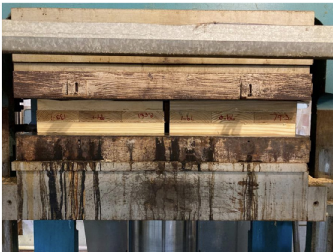
Figure 1. Panels in Dieffenbacher laboratory hydraulic press.
