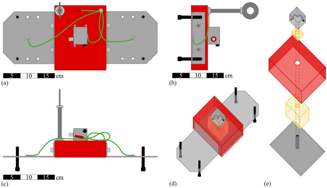
Figure 1. Continuous surface charge detection device (a) top view, (b) elevation view, (c) side view, (d) 3D model, and (e) elements of the measuring box with the dimensions of  $15 \times 20$  cm (top to bottom): connector head to attach the EFM, insulating polytetrafluoroethylene cube, Faraday casing, insulating polymer cube, and detection plate – connected to the top box along the dotted lines. EFM, electric fieldmeter.
