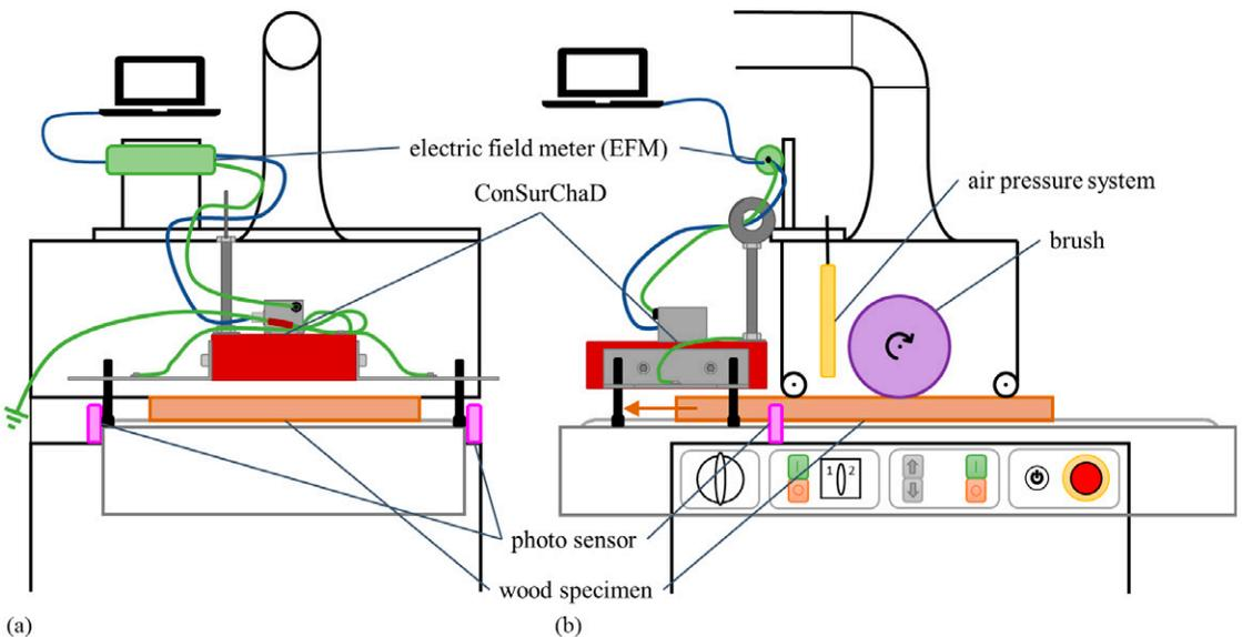
Figure 3. An experimental setup was used to measure the surface charges of wood samples caused by surface brushing: (a) side view and (b) elevational view. ConSurChaD, continuous surface charge detection.
