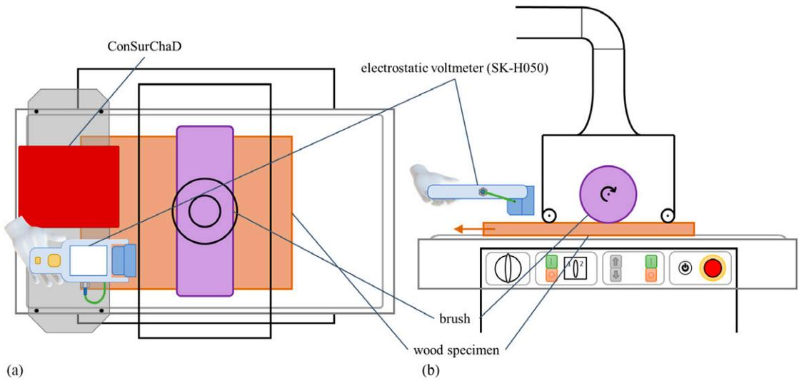
Figure 4. The top view of simultaneous measurement shows the ConSurChaD device and the Keyence SK-H050 reference (a); the elevational view of the brushing machine with the surface-charge measurement, with the installed Keyence device (b). ConSurChaD, continuous surface charge detection.
