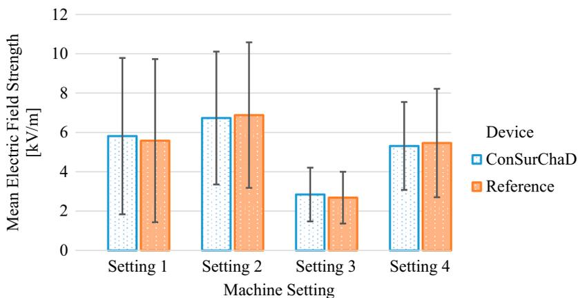
Figure 6. Comparison of electric field strength measurements with the newly developed ConSurChaD device, compared with the Keyence SK-H050 reference. Mean and standard deviations of electric field strength in kV/m are shown, using the machine setting high brush pressure and fast feed rate (1); high brush pressure and slow feed rate (2); low brush pressure and fast feed rate (3); and low brush pressure and slow feed rate (4) ( $n = 15$ ). ConSurChaD, continuous surface charge detection.
