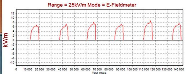
Figure 5. Setup (left) and data plot as produced with the readout software (right) plotting the electric field strength [kV/m] of three samples getting brushed twice.
