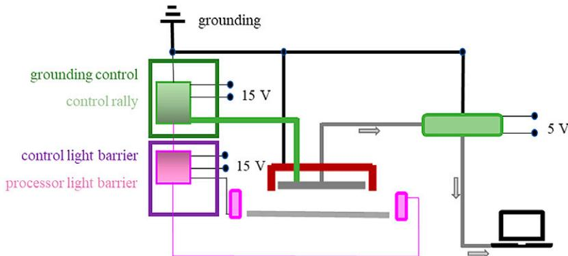
Figure 2. Electrical circuits of the continuous surface charge detection device.
