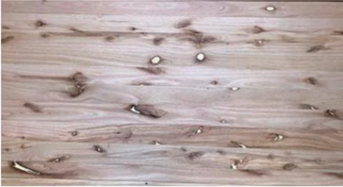
F<sub>6</sub>: 6 mm thick fibre *E. nitens* glued to marine ply substrate and veneer backing
