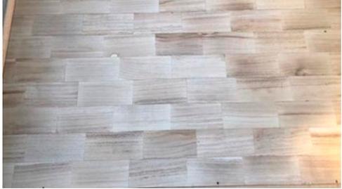
D<sub>12</sub>: 12 mm thick solid, densified *E. nitens*
