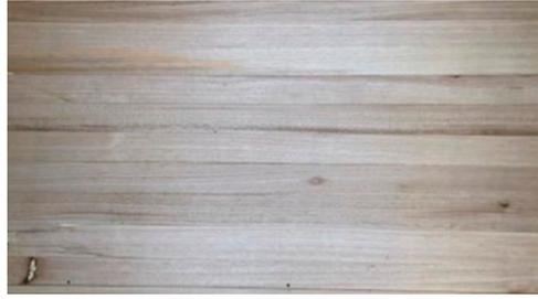
S<sub>6b</sub>: 6 mm thick sawlog *E. nitens* glued to marine ply substrate
