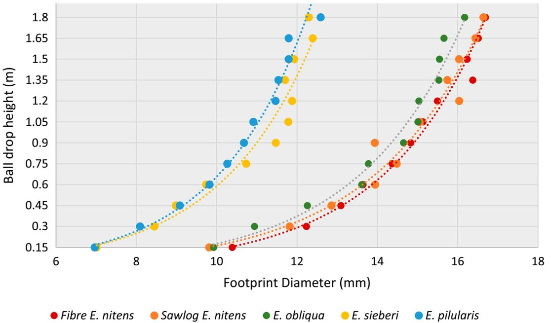
Figure 6. Footprint diameter with different drop heights.
