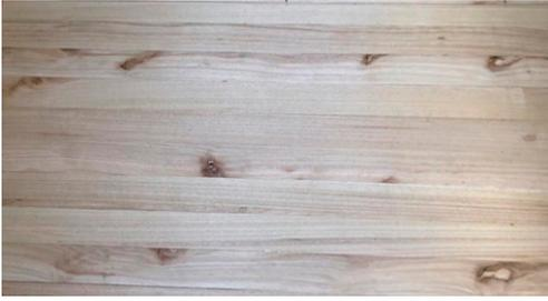
S<sub>6a</sub>: 6 mm thick sawlog *E. nitens* glued to marine ply substrate and veneer backing
