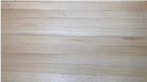
S<sub>1.2mp</sub>: 1.2 mm thick sawlog *E. nitens* glued to marine ply substrate and veneer backing
