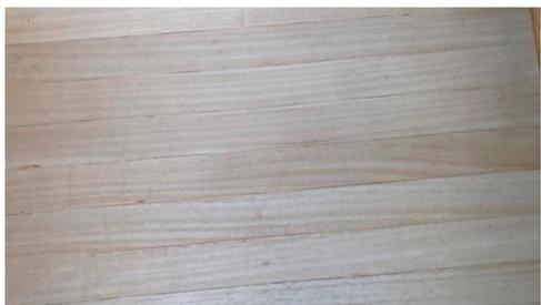
S<sub>1.2np</sub>: 1.2 mm thick sawlog *E. nitens* glued to *E. nitens* ply substrate and veneer backing
