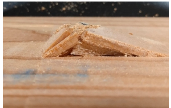
Figure 11. Typical withdrawal failure mode showing pull out of uppermost layer on specimen K.F.CLT-A_2.
