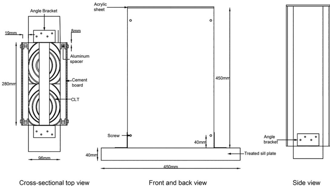
Figure 2. 2D drawing of a CLT envelope specimen.
