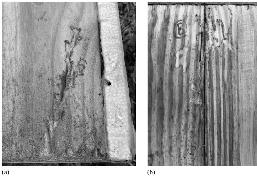
Figure 6. Damage (a) from a typical control specimen and (b) in one Termimesh specimen, where termites had constructed a mud tube from the soil line up to the top of the panel and attacked the wood at the top of the CLT.
