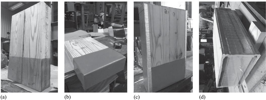
Figure 3. Envelope installation (a) CLT with Termimesh barrier, (b) CLT with Obex11 barrier, (c) CLT edges sealed with aluminum tape, and (d) a complete CLT envelope specimen with spacers and cement board cladding.
