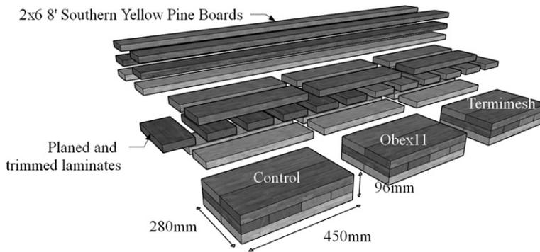
Figure 1. Lumber layout to manufacture one batch of cross laminated timber (CLT) specimens.
