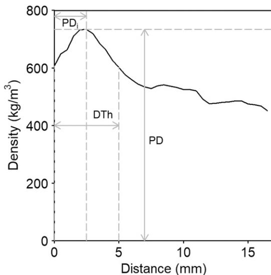
Figure 3. Metrics calculated to characterize the one-dimensional density profiles.
