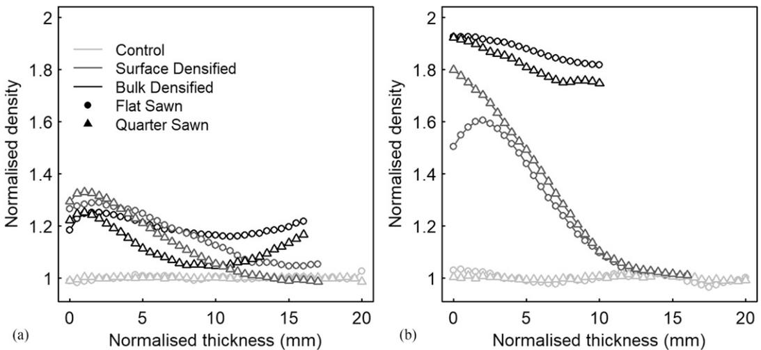
Figure 6. Average density profiles for *E. Fastigata* (a) and *E. Nitens* (b). The normalized density is based on the pretest density of each board. The normalized thickness is based on the target thickness for each densification process.
