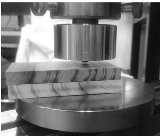
Figure 2. Brinell hardness testing set up, showing the sample to be tested sitting on top of a second sample of the same species, grain orientation, and densification process (ie, surface- or bulk-densified).
