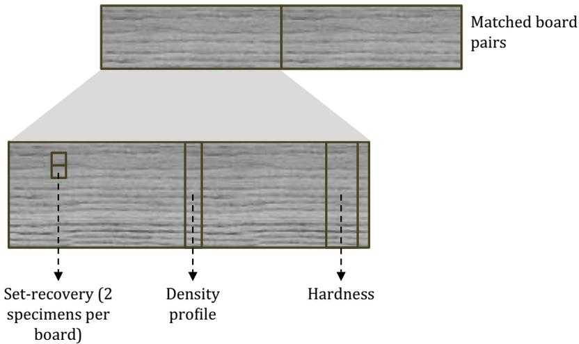
Figure 1. A cutting plan showing the location of the property test specimens within each board. The view is of the upper face of the board.
