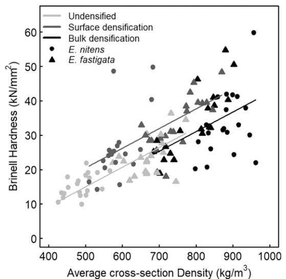
Figure 7. Relationship between final density and Brinell hardness for each species and densification type. *E. Fastigata* is shown by triangles, *E. Nitens* by circles. The best fit lines show a correlation between density and hardness, taking the densification process into account. Adjusted  $R^2 = 0.586$ ,  $p < 0.001$ .
