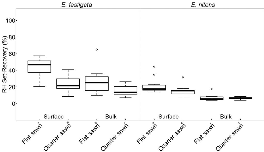
Figure 5. RH-cycling set-recovery by densification type, species, and grain orientation. Superscript letters indicate treatments within each species that are not significantly different from each other (95% confidence level, Kruskal-Wallis test with Holm adjustment).
