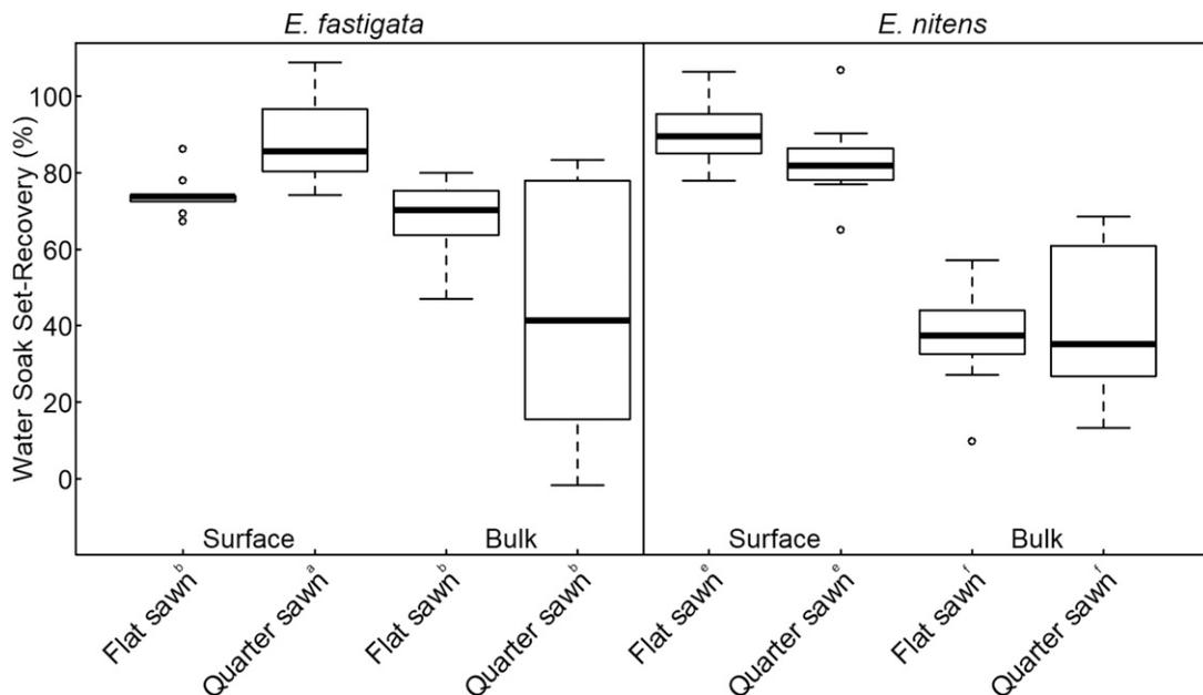
Figure 4. Set-recovery by densification type, species, and grain orientation. Superscript letters indicate treatments within each species that are not significantly different from each other (95% confidence level, Kruskal-Wallis test with Holm adjustment).
