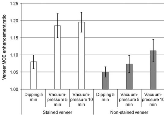
Figure 4. Enhancement of veneer dynamic modulus of elasticity (MOE) from 5-min dipping and vacuum-pressure treatments.
