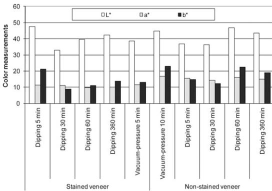
Figure 6. Color components of laminated veneer lumber billets made from veneer with different treatments.
