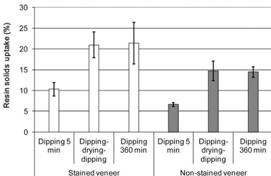
Figure 2. Comparison of resin solids uptakes for stained and unstained veneers among the three dipping times.
