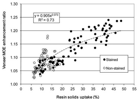
Figure 3. Correlation between veneer modulus of elasticity (MOE) enhancement and resin solids uptake.
