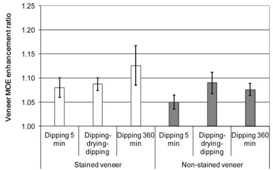
Figure 5. Enhancement of veneer dynamic modulus of elasticity (MOE) from different dipping treatments.
