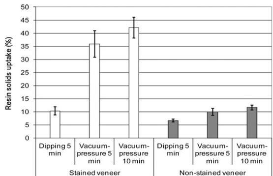
Figure 1. Effect of treatments on resin solids uptake for stained and nonstained veneers.
