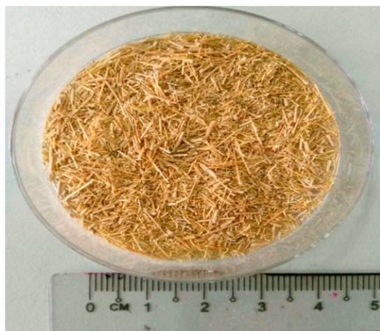
Figure 2. Ground bamboo specimen (40 mesh) used for analysis.
