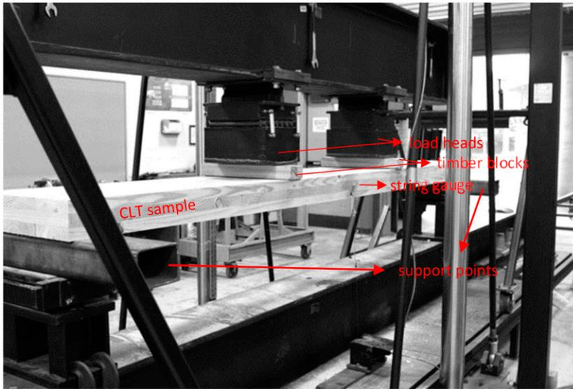
Figure 1. Test setup.
