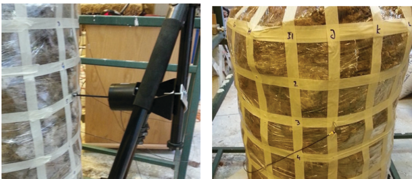
Figure 2. Pictures over details of the experimental measurement setup on the palm tree log. Left: Attachment of shaker, for force excitation. Right: Attachment of accelerometer, for response signal recording.
