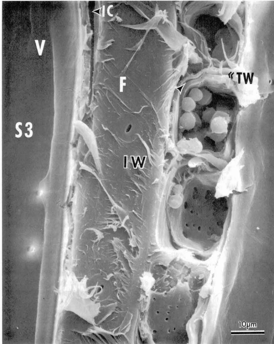
FIG. 1. In this micrograph of sweetgum that failed in tangential shear, both transwall (TW) and intrawall (IW) failure can be noted in adjoining cells. The ray parenchyma cell wall has delaminated (arrow). The lumen lining layers (S3) appear to be intact in cells at both right and left extreme edges of this micrograph. Intercell failure appears at upper center at the vessel and fiber interface.
