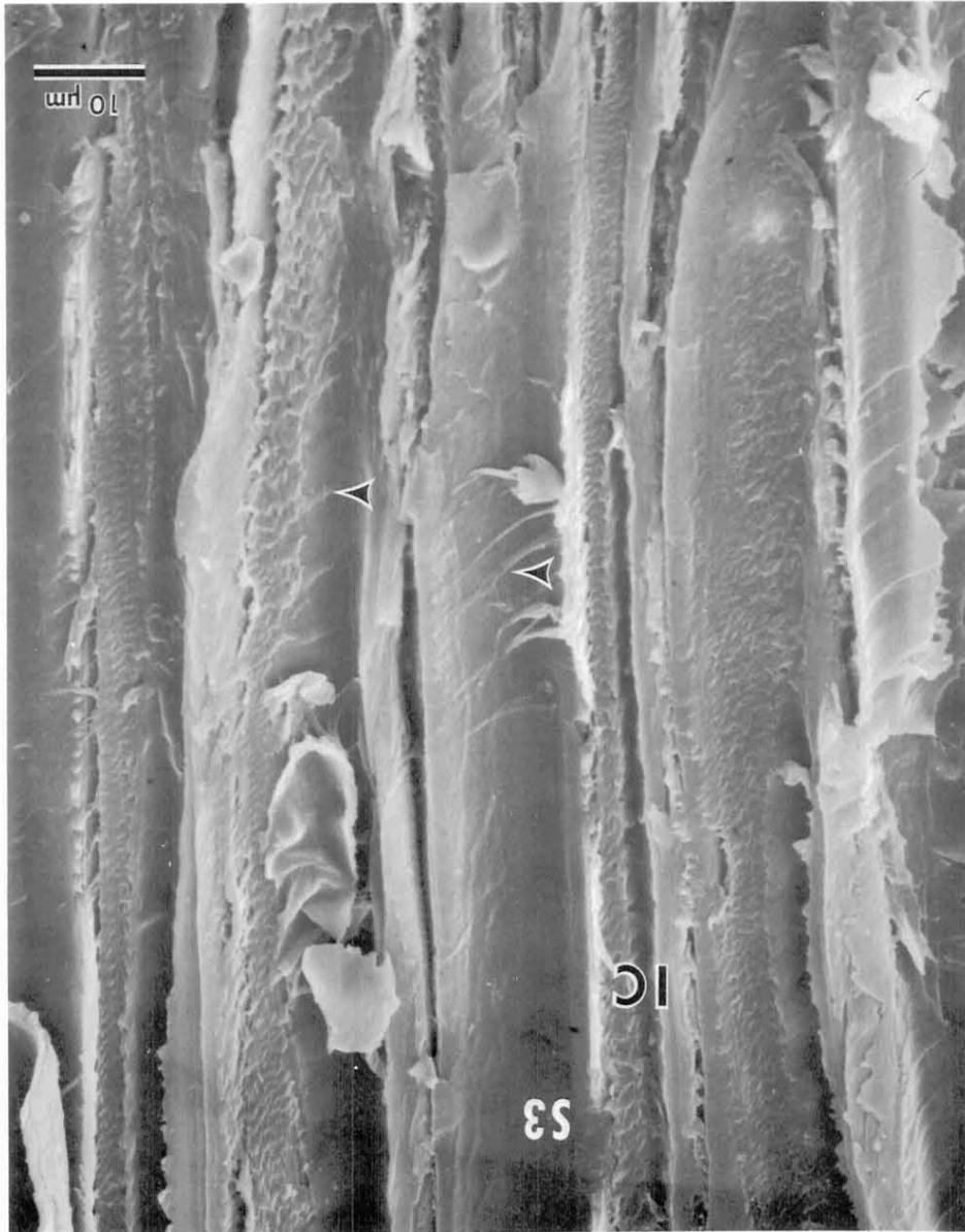
FIG. 4. Hickory compression specimen which exhibits cell-wall deformations visible in the lumens, separation of fibers at or near the middle lamella and intrawall failure. Arrows indicate S3 deformations.
