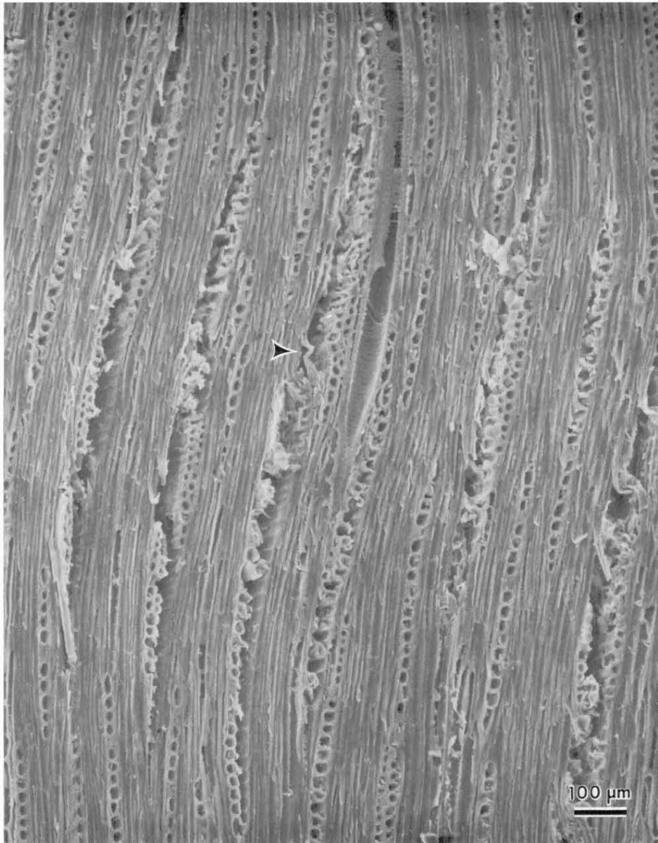
FIG. 2. Tangential surface of red oak compression test specimen showing the start of gross buckling and the initiation of separation in the vicinity of rays. Intercell failure proceeds above or below the rays, but appears to have started at fiber/ray interface in most cases. Arrow indicates area enlarged in Fig. 3.
