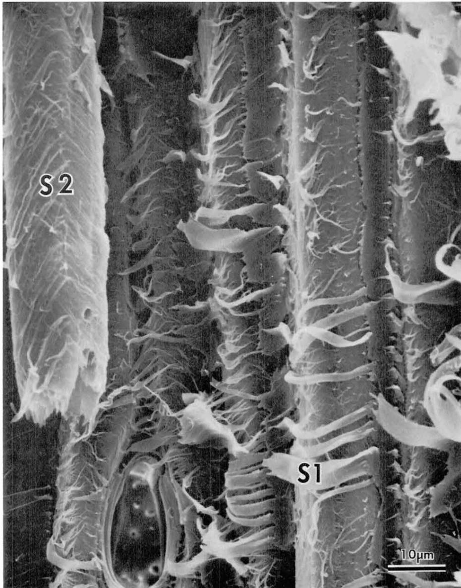
FIG. 10. Intrawall failure predominates in the thick-walled cells of this hickory specimen that failed in tangential shear. The S2 and the S1 are the more prominent layers visible in this micrograph. Intrawall failure takes place within either the S1 or the S2, or at their interface, the S1/S2. The single ray parenchyma cell, lower left, exhibits transwall fracture.
