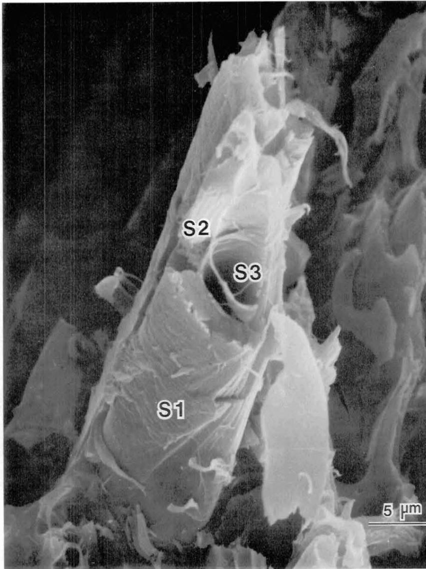
FIG. 19. These fibers in a tensile test specimen of hickory exhibit intrawall failure in which all three secondary wall layers can be identified through their orientation. Obviously transwall failure occurred ultimately as well.
