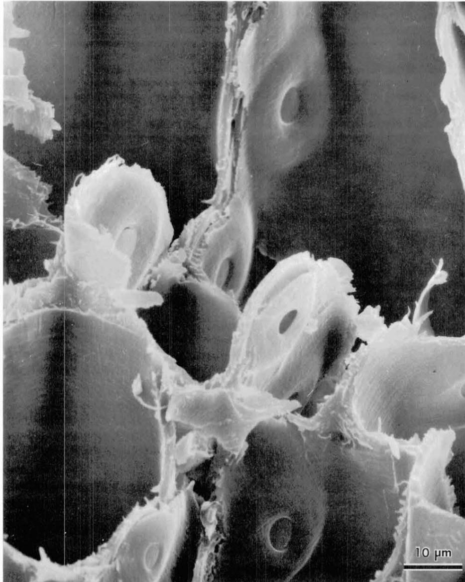
FIG. 23. Although much as been mentioned in the literature about the role of bordered pits in cell-wall failure in conifers, this is one of the few clear examples of their resistance to transwall failure. Instead, the fracture lines in these earlywood tracheids of southern pine follow the rim or annulus of the bordered pit pairs in several cases.
