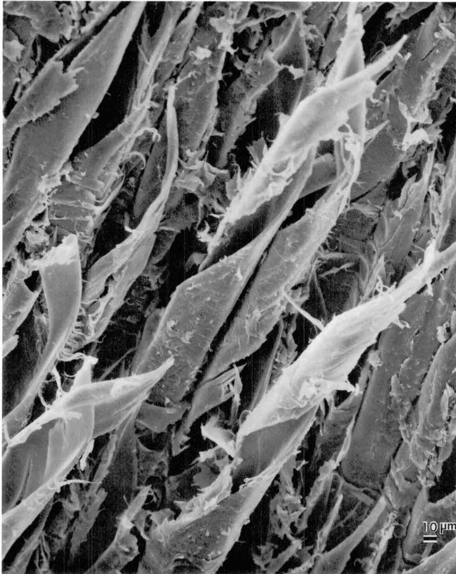
FIG. 25. In this example of southern pine latewood that failed in tension, evidently the S2 layers pulled out of the S1, which would presumably be found in the matching end of the test specimen. The unwinding phenomenon seen in both hardwoods and softwoods is found throughout this fracture surface and consists of S2 with only traces of the other layers.
