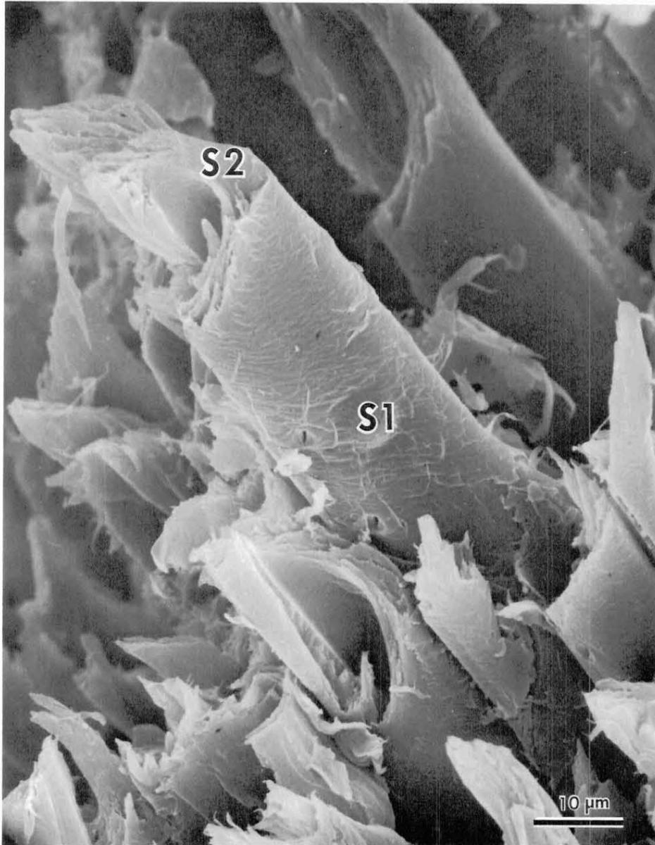
FIG. 18. In a wood of higher specific gravity such as red oak, tensile test specimens break with a less "brash" type of failure. Many individual fibers extend out of the failure zone. Clearly, intrawall failure predominates as S1 and S2 microfibrillar orientation can be seen throughout the micrograph.
