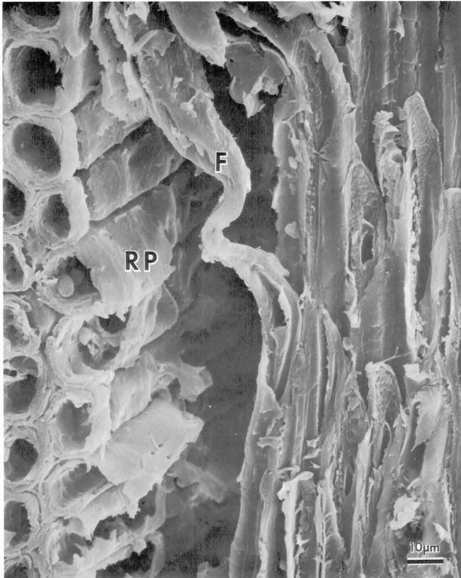
FIG. 3. Area indicated by arrow in Fig. 2 was recorded after inverting the compression test specimen and increasing the magnification approximately tenfold. The buckling of fibers and the separation of fibers from the ray parenchyma tissue in intercell failure are emphasized.
