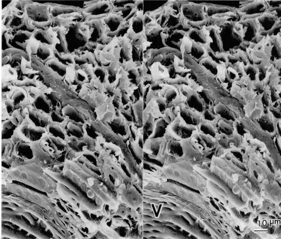
FIG. 21. In this stereo pair of a red oak tensile test specimen, an area from the earlywood has been selected to illustrate the abrupt transwall failure of the fibers as well as the vessel wall. Very few traces of long projections of cell wall can be found.
