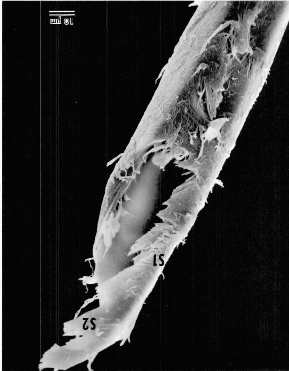
Fig. 22. This is an apparently unsplit portion of a southern pine latewood tracheid that failed in tension. The tendency of the S2 to unwind can be seen, while portions of the S1 with its nearly horizontal orientation of microfibrils remain.
