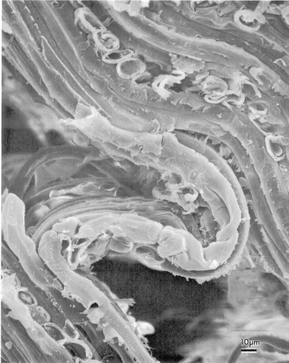
FIG. 5. Tangential view of a sweetgum specimen tested in compression parallel to the grain. The extreme buckling even at this microscopic level results from separation of cells above and below the buckling zone. Both intercell and intrawall failure can be seen in this micrograph.
