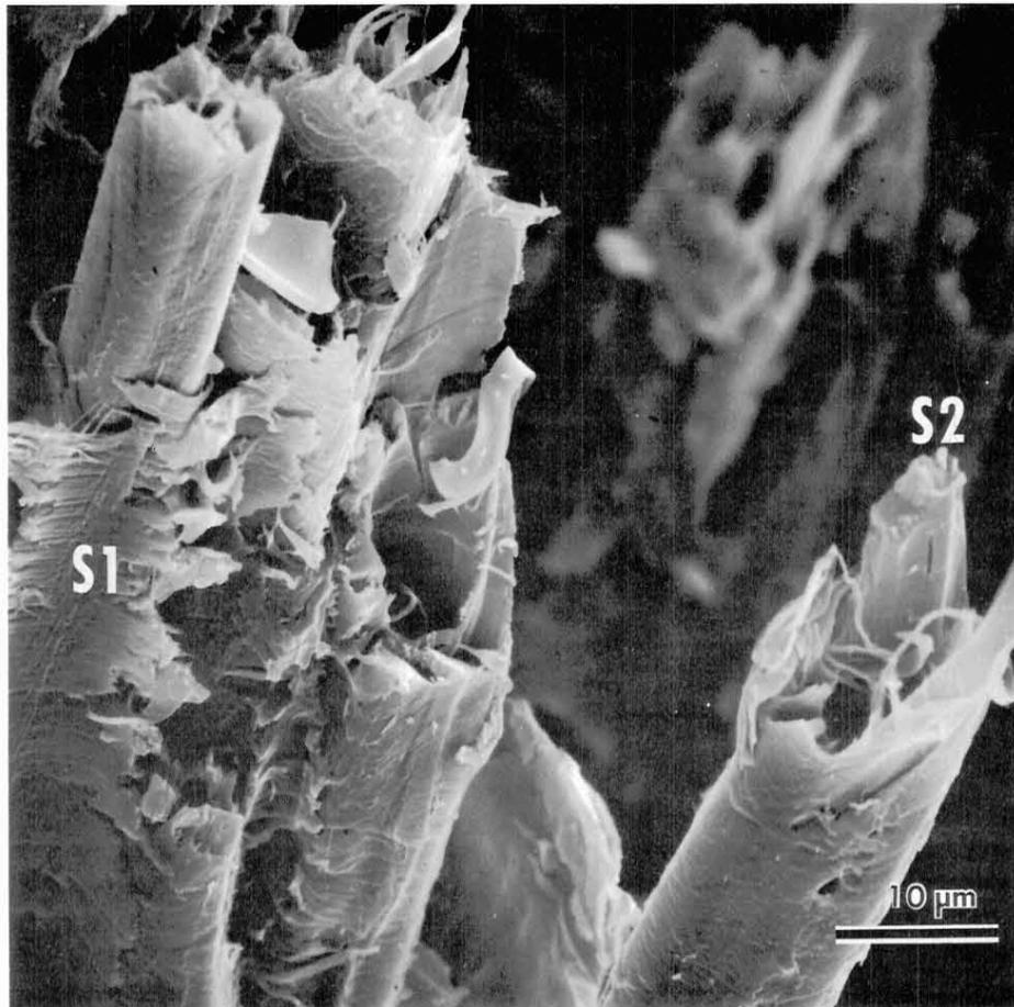
FIG. 20. The unwinding phenomenon discussed in the text appears in this specimen of hickory tested in tension parallel to the grain, as it has in several other instances. Intrawall failure at the S1/S2 predominates, while transwall failure is most evident at the S2 regions of the cell walls.
