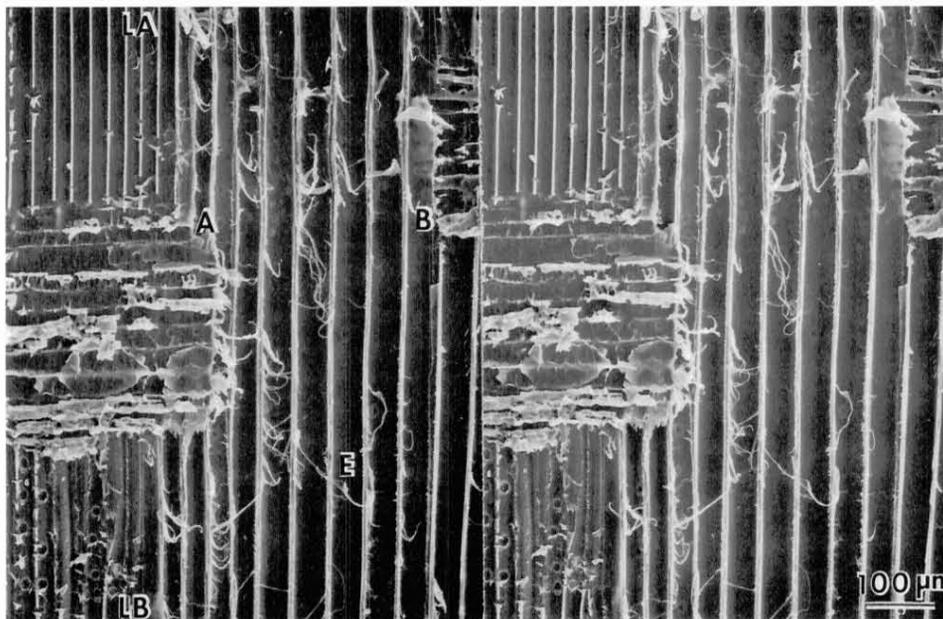
FIG. 15. Radial shear in southern pine, when viewed at low magnification, reinforces the concept of cell-wall thickness as the determining factor leading to intrawall vs. transwall failure. This stereo pair makes it easier to compare the fracture zones in earlywood (E) and latewood (LA and LB).
