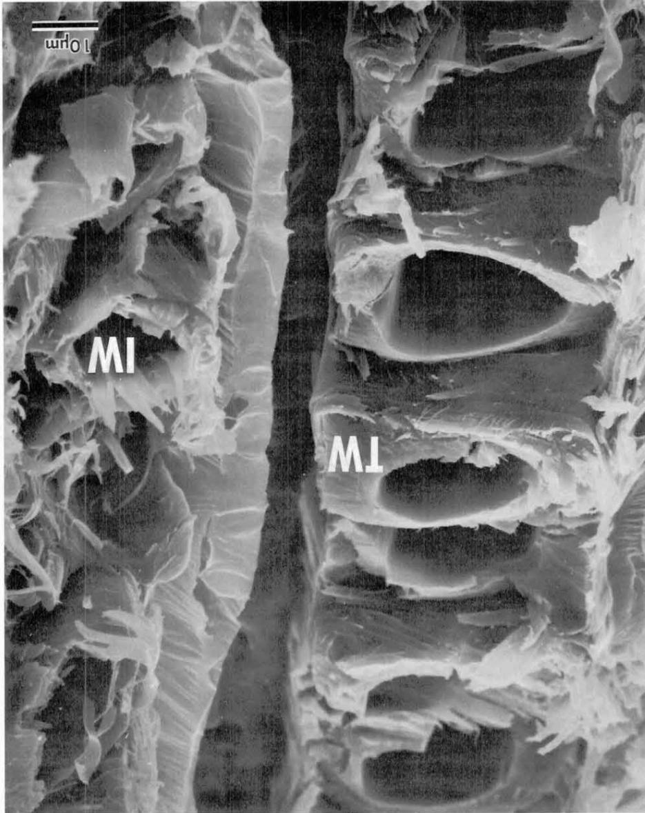
Fig. 24. On the left side of this micrograph, there is a row of thick-walled tracheids in the latewood of southern pine. All show abrupt transwall failure, while those on the other side of the ray that traverses the center of the micrograph from top to bottom exhibit more intrawall failure. It appears likely that the distribution of anatomical components influences tensile tests such as this just as it does in shear and compression tests.
