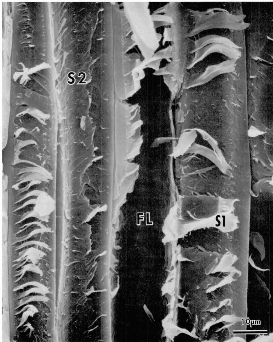
FIG. 11. A fracture surface very similar to that in Fig. 10 is produced in radial shear testing as in this red oak specimen. Intrawall failure of the longitudinal elements involves the S1 or the S2, or their mutual interface. This micrograph resembles that of Fig. 10 except that one fiber lumen was left intact (center), presumably because of transwall failure.
