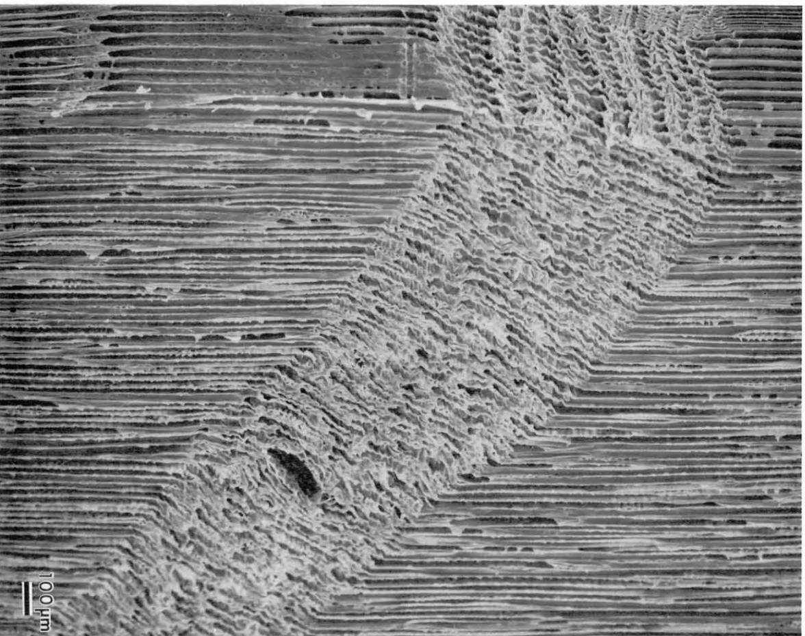
FIG. 7. The failure lines resulting from compression parallel to the grain are distinct in softwoods such as this sample of southern pine, which is mostly earlywood, because of the relatively simpler anatomical structure. The characteristic 45° to 60° angle made by the failure line with the axial direction of the wood is apparent even at this magnification.
