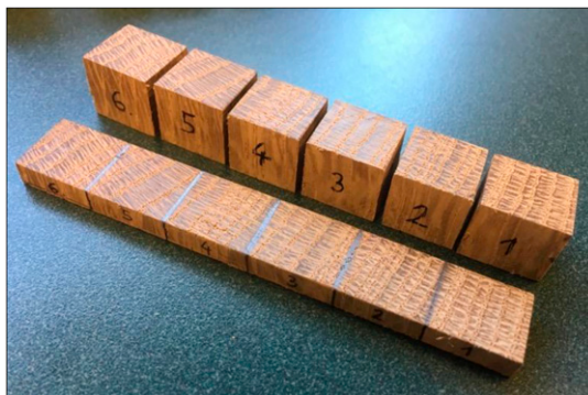
Figure 2. Photo of a prepared specimen sample showing the six sections marked on the strip and the six matching sample cubes. The cubes were cut from wood immediately below the strip samples (separated only by the 2 mm of wood removed by the saw blade).
