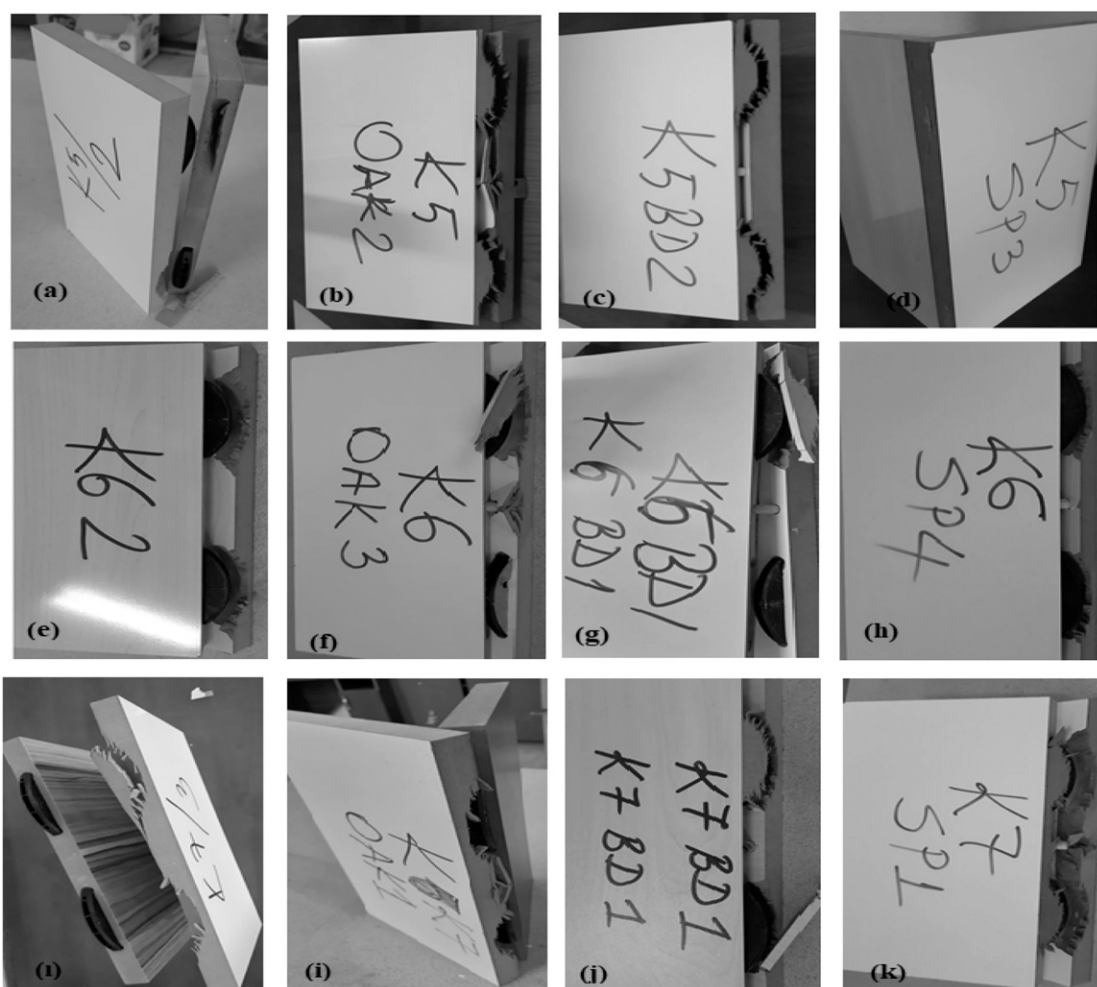
Figure 10. Types of deformation of L-type corner joints resulting from the compression test; 50 mm end distance + control (nondowel) (a), 50 mm end distance + oak dowel (b), 50 mm end distance + oriental beech dowel (c), 50 mm end distance + scotch pine dowel (d), 60 mm end distance + control (nondowel) (e), 60 mm end distance + oak dowel (f), 60 mm end distance + oriental beech dowel (g), 60 mm end distance + scotch pine dowel (h), 70 mm end distance + control (nondowel) (i), 70 mm end distance + oak dowel (j), 70 mm end distance + oriental beech dowel (k), and 70 mm end distance + scotch pine dowel (l).
