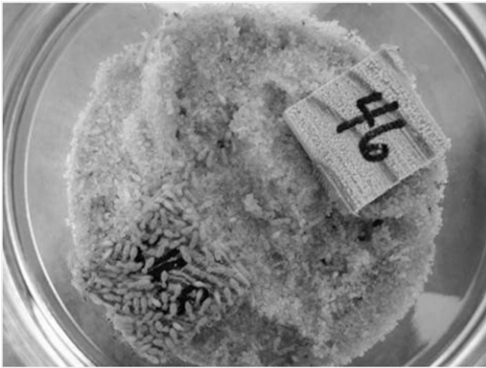
Figure 2. Example of workers aggregating on a higher specific gravity sample 2 h after introduction to a choice test (Note how FST are attracted to the high SG sample, while avoiding the low SG sample).
