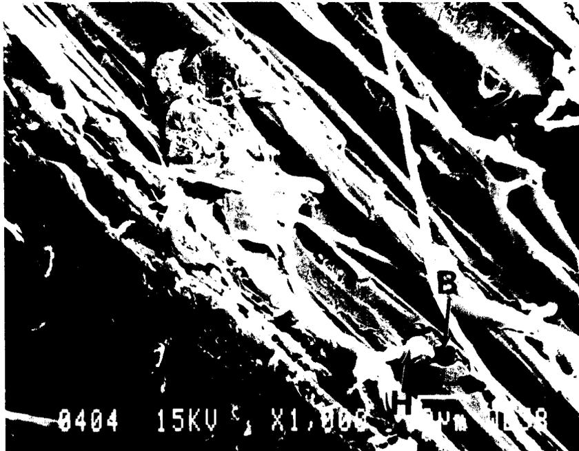
Fig. 5. A bore hole (B) produced by a fungal hypha (H) at the chip surface. ( $\times 1,000$ )
