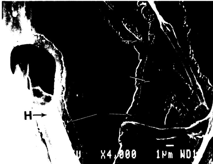
FIG. 7. Erosion troughs (E) produced by enzymes secreted by (collapsed) fungal hyphae (H) lying in the centers of the troughs. ( $\times 4,000$ )
