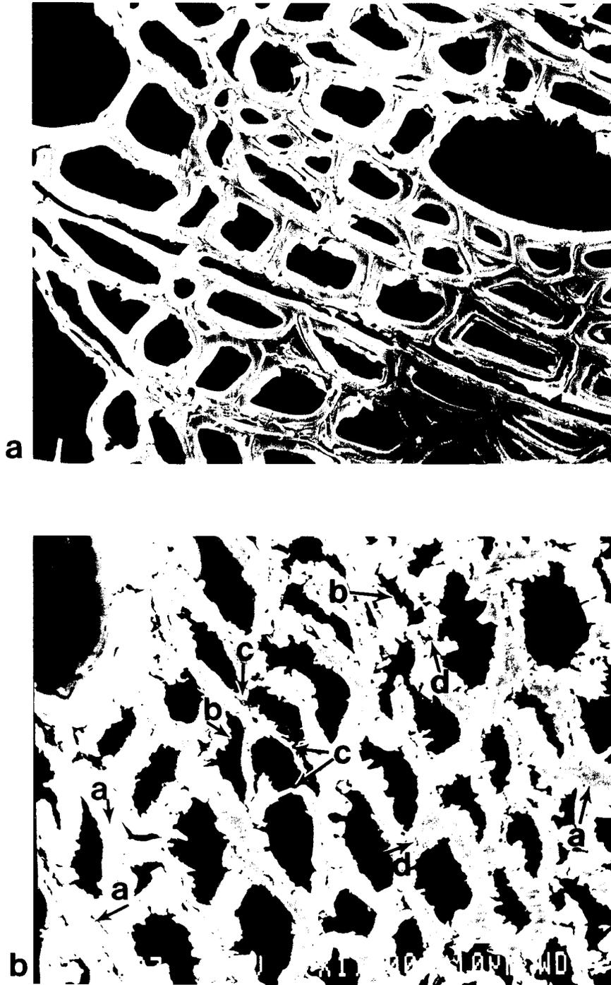
FIG. 10. The normally rigid wood cell wall structure within an aspen chip (A) was modified by the model 3-week fungal treatment used in the bench-scale biomechanical pulping process. (B) Modifications included (1) cell wall swelling (a), (2) enzymatic softening or relaxing resulting in the partial collapse of the tubelike-cell structure (b), and (3) localized areas of wall thinning (c) or fragmentation (d). ( $\times 1,000$ )
