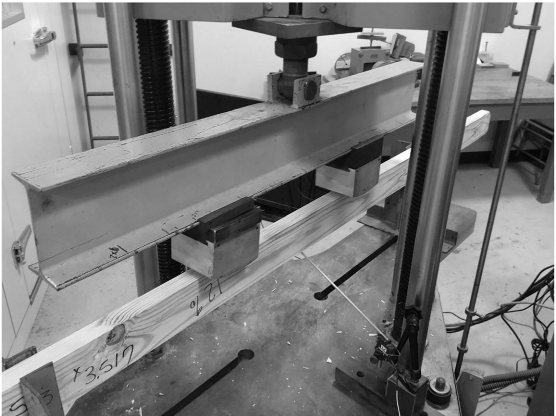
Figure 1. A southern pine 2 × 4 undergoing a static bending test per ASTM D 198-15, flexure method.
