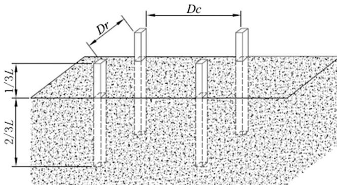
Figure 1. Detailed schedule of stakes for field exposure test.
