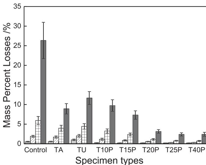
Figure 3. Mass loss caused by brown-rot fungus *Gloeophyllum trabeum* (Pers.) Murrill CFCC 86617 at 3-wk intervals during laboratory tests (Note: The light gray, diagonal, gridded, and black columns expressed mass losses after 3-, 6-, 9-, and 12-wk tests, respectively). CFCC, China Forestry Culture Collection Center.
