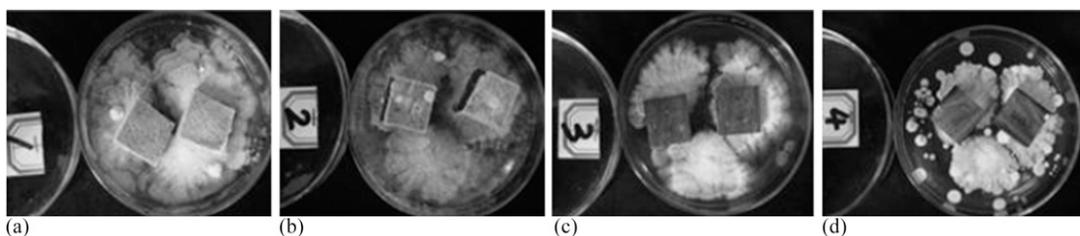
Figure 4. Typical specimen after 12-wk incubation in laboratory test. (a) Control group, (b) ACQ specimen, (c) urea-formaldehyde specimens, and (d) 20% phenol-formaldehyde specimens.
