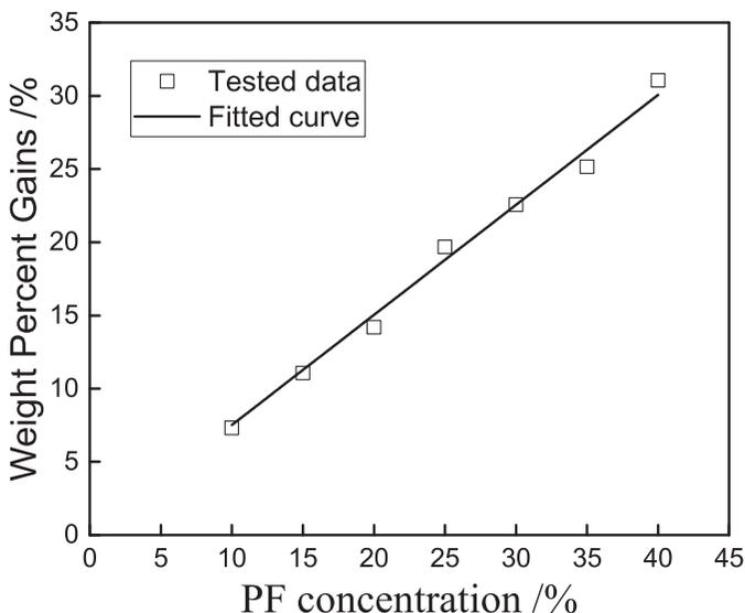
Figure 2. Curves of weight percent gains in phenol–formaldehyde (PF) specimens with resin concentration. The goodness of fit values was 0.9907.
