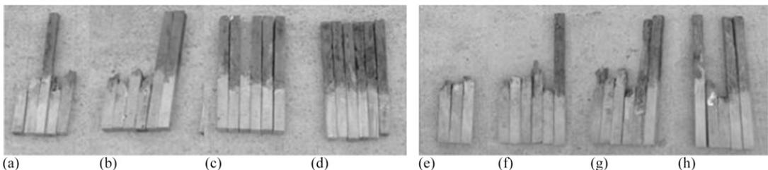
Figure 5. Decayed specimen after field stake test. (a-d) Decayed specimens after the 12-mo test and (e-h) decayed specimens after the 24-mo test (Note: (a) and (e) Control group; (b) and (f) ACQ specimen; (c) and (g) urea-formaldehyde specimens; and (d) and (h) 20% phenol-formaldehyde specimens).
