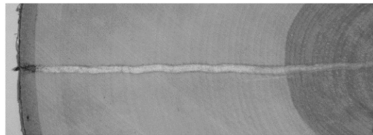
Figure 8. Bore channel observed in one of the drillings made on a green yellow birch ( Betula alleghaniensis ) log.
