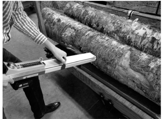
Figure 1. Drilling resistance measurements on a yellow birch log.
