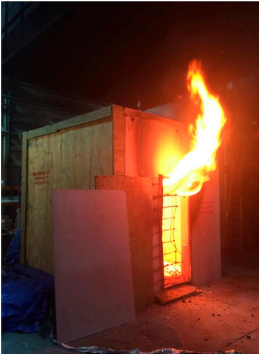
Figure 2. Exposed cross-laminated timber compartment fire test undertaken at BRE by the University of Edinburgh and Arup (image, Arup).
