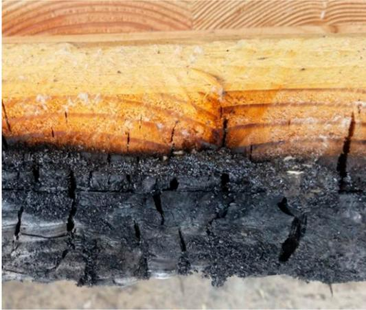
Figure 8. Cut section through five-ply cross-laminated timber floor panel, successfully passing a fire test to ASTM E119 to 2 h, without any delamination occurring (image, Arup).
