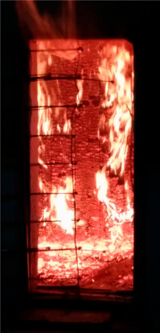
Figure 3. Cross-laminated timber with delamination occurring at ply interface (dark areas on wall) during fire test (image, Arup).
