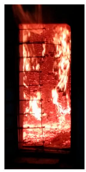
Figure 3. Cross-laminated timber with delamination occurring at ply interface (dark areas on wall) during fire test (image, Arup).
