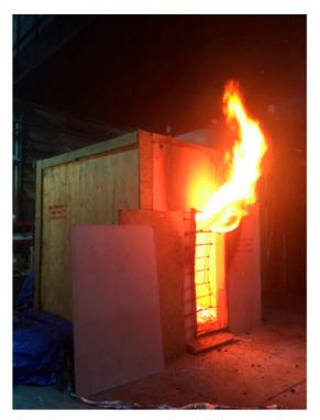
Figure 2. Exposed cross-laminated timber compartment fire test undertaken at BRE by the University of Edinburgh and Arup (image, Arup).
