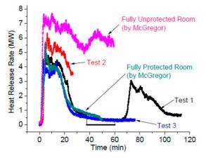
Figure 7. Results from Medina and McGregor, showing the difference in fire size (heat release rate) for a cross-laminated timber (CLT) room with full gypsum protection, one CLT wall exposed (Tests 3), two walls exposed (Tests 1 and 2), and all walls exposed (Medina 2014).
