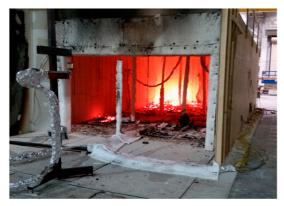
Figure 4. Fire Protection Research Foundation fire Test 2, near completion at 100 min after ignition (image, Arup).
