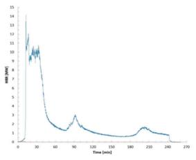
Figure 5. Heat release rate curve from Test 3 (preliminary only) (Kimball et al 2017).
