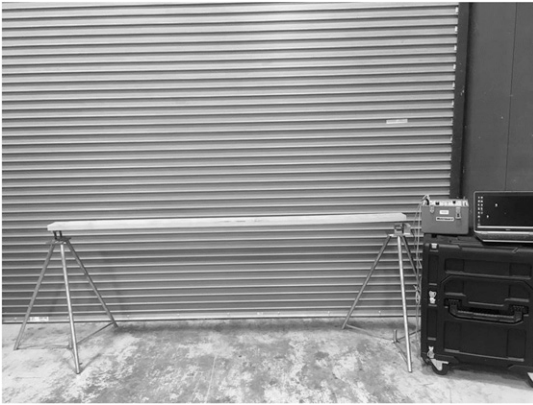
Figure 2. Transverse vibration technique: Metriguard E-computer model 340 (edgewise–flatwise).
