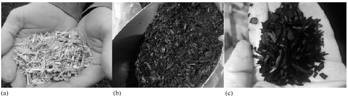
Figure 2. Wood feedstock to final product conversion—(a) microchips made from the wood of coniferous tree species; (b) biochar from wood chips carbonized in a pyrolysis system; and (c) activated carbon made from biochar activated using steam in a rotary calciner.
