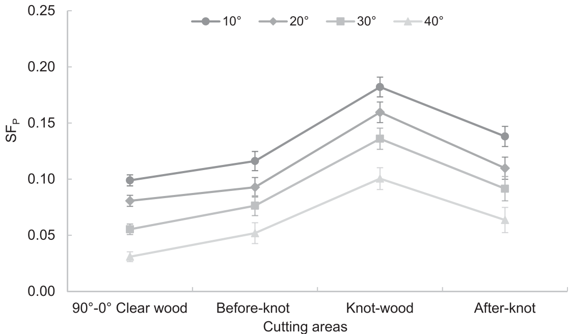
Figure 6. Specific parallel force mean as a function of the cutting area for all rake angles (bars correspond to the standard error).
