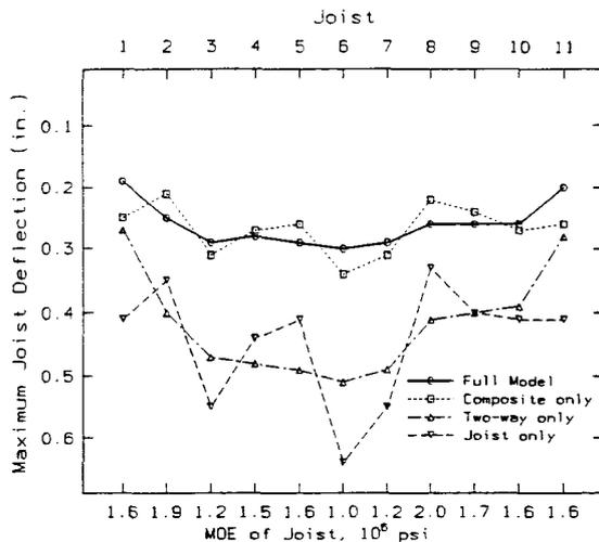
FIG. 1. Patterns of joist midspan deflections of a floor with variable joist stiffnesses, uniform load (from Criswell 1981).
