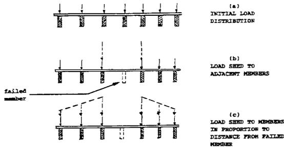
FIG. 2. Load redistribution schemes for system with flexible deck.
