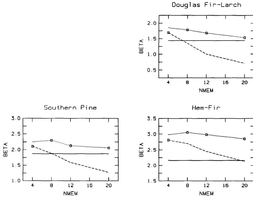
FIG. 6. Comparison of limit state definitions ..... 2 Adjacent --- Any 2 □ Composite — Single-member.
