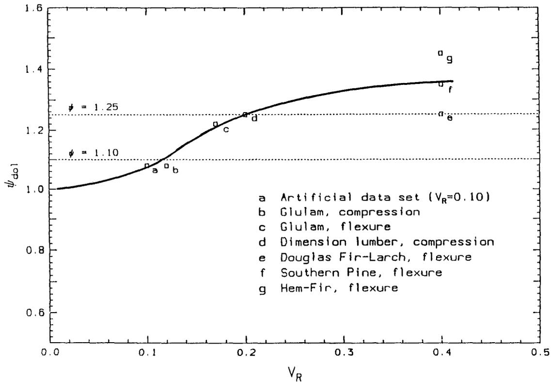
Fig. 8. Comparison of system factors for different lumber types and limit states.
