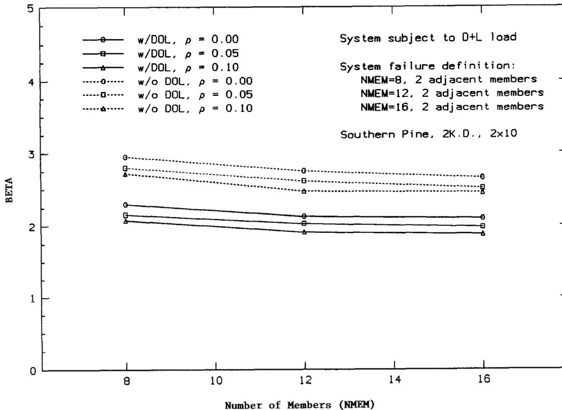
FIG. 7. Effect of increasing ( $\rho_{R,R}$ ) on system reliability.
