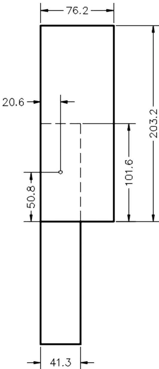
Figure 2. Schematic of connection (all dimensions in mm).
