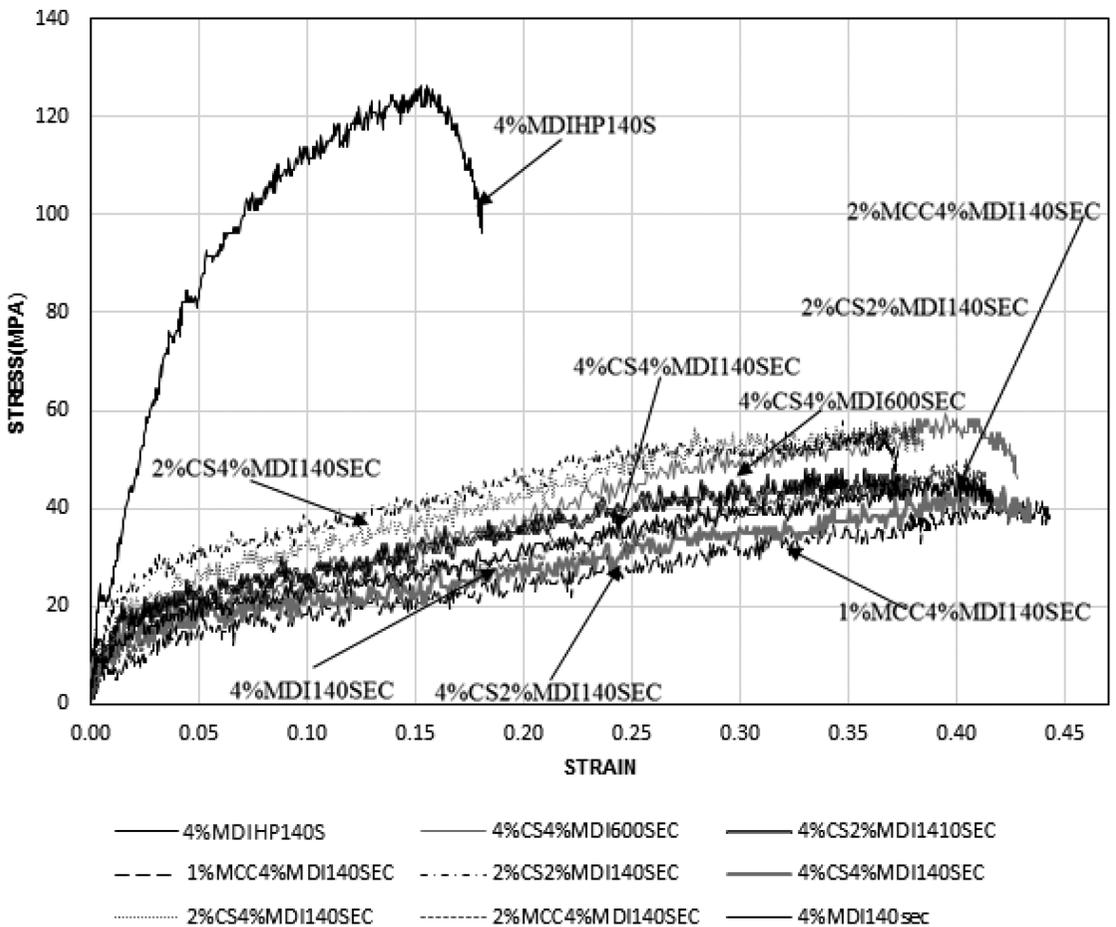
Figure 4. Dynamic stress-strain curve of wood-based biocomposites at 20 psi (strain rate from 766 to 1587 s<sup>-1</sup>).
