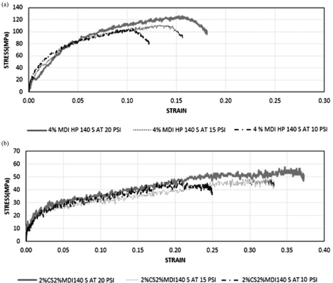
Figure 5. Effect of strain rate on wood-based biocomposites. (a) Effect of strain rate on 4%MDIHP140S; (b) effect of strain rate on 2%CS2%MDI140S.
