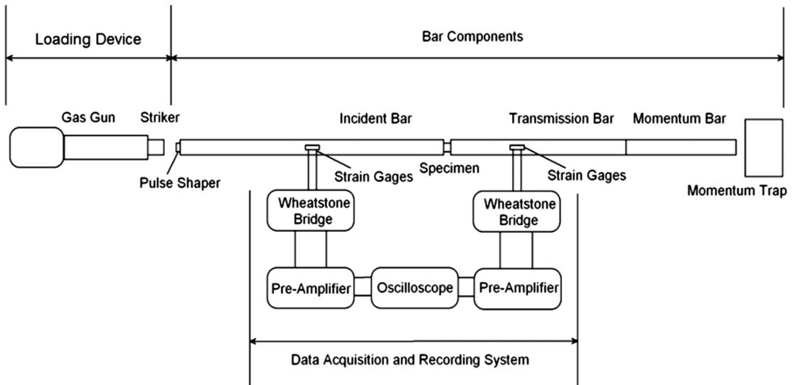
Figure 1. Split-Hopkinson bar (Kolsky) diagram: device located at the University of Mississippi (Ramesh, 2008).
