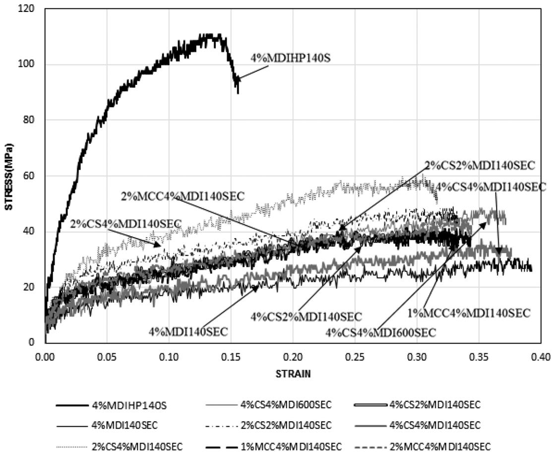
Figure 3. Dynamic stress-strain curve of wood-based biocomposites at 15 psi (strain rate from 727 to 1380 s<sup>-1</sup>).
