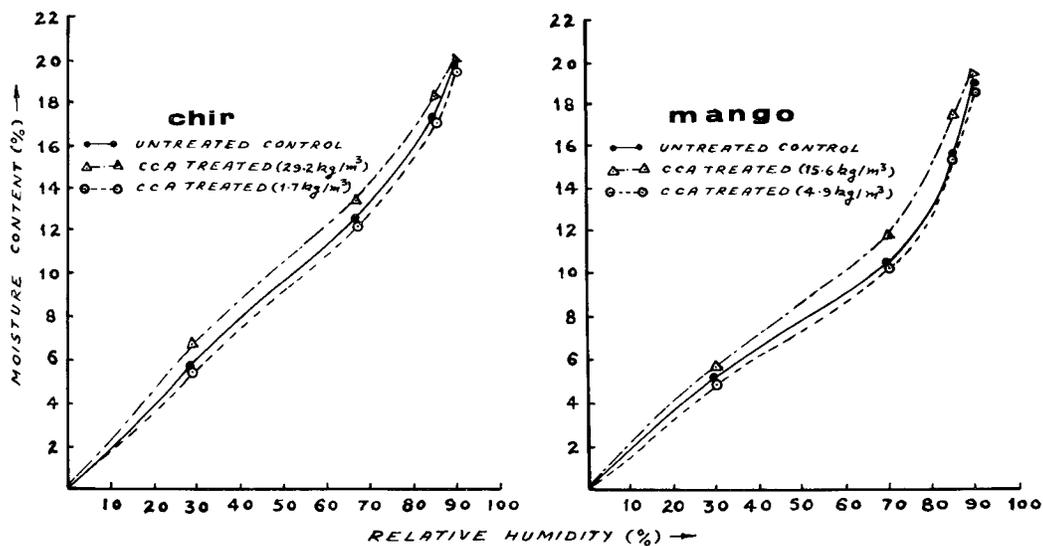
FIG. 1. Sorption curves for treated and untreated chir and mango wood.
