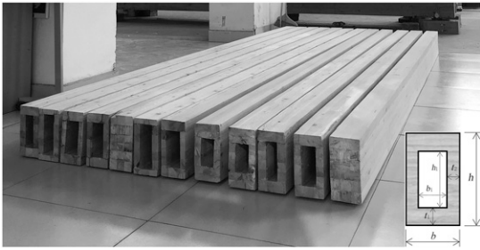
Figure 1. Hollow glulam beam.
