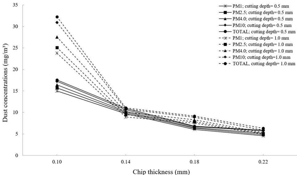
Figure 2. Adjusted dust concentrations as a function of average chip thickness for particle size fractions.
