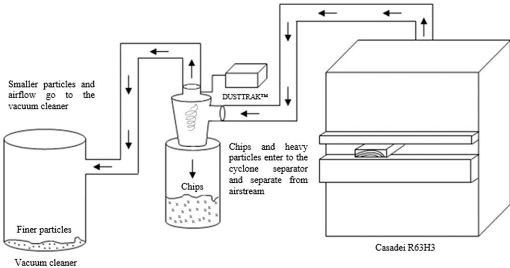
Figure 1. Dust measurement system used during machining treatments.
