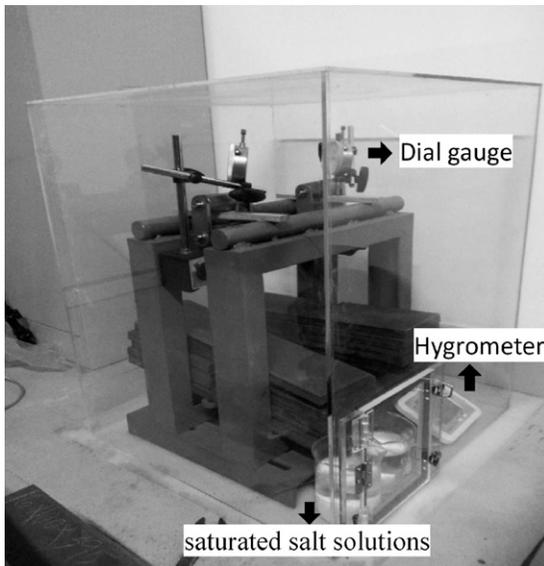
Figure 1. The laboratory-made device of MS creep test.
