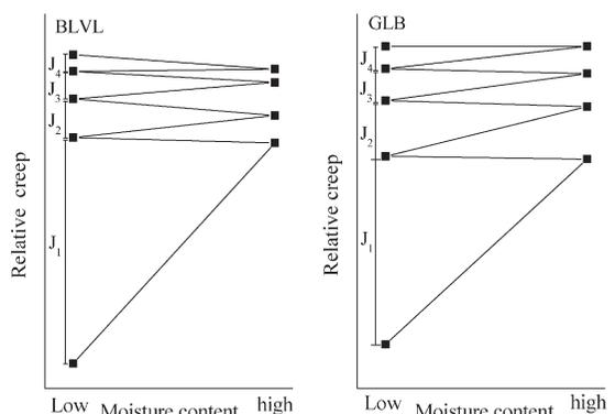
Figure 6. The relationship of moisture and relative creep.
