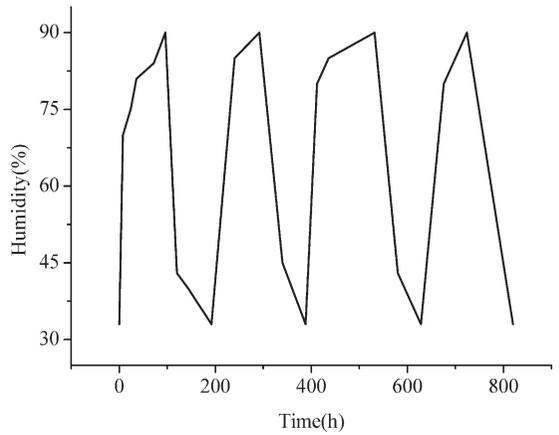
Figure 2. The humidity fluctuation of MS test.
